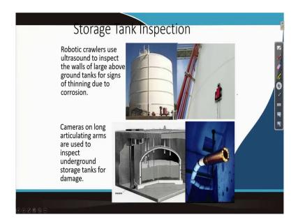
Similarly, you are in a storage tank. There also if you can go for nondestructive testing because you cannot take these things out of service, you can go on testing like this. Similarly, your that whenever you are using in a area which are very critical any failure may give raise to a major problem should be brought under nondestructive testings.
