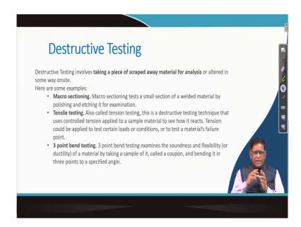
Now, in the destructive testing you may be knowing that what need to be done. If suppose you have done a welding, after that welding things are correct or not you need to do a micro sectioning test. A small section or portions are cut and taken it out and then they will be doing over there some testings are done.
