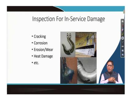
So, that in service for in the mining industry also you will find that is a crack detections for your corrosion detections for your erosion and wear detections, heat damage those things need to be find out. You can see here that these are the your damage due to the erosion, corrosions.
