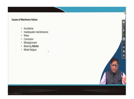
So, the other is this cause of the failure must be identified that whether it is by accident, whether it is because of inadequate maintenance, because of wear or because of corrosion misalignment or bearing failure or metal fatigue. These are the now, you need to study these items separately and for that you will have to find out you just write down these words start, study in the internet find out that.
