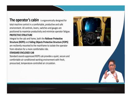
So, that the material is retained within the truck body. So, that type of safety systems are there the operator's cabin as it said your roll over protective structures ROPS and falling object protective structures. These two are given and that operator cabin is high pressurized. So, that there should not be acoustically treated. So, you will not because in underground metal mine when there are lot of drills and all will be working it will be very noisy.
