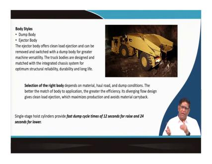
So, this 2 types of one is your just dumping by the rear ditchers and another is by ejector type of things are there and then for a operations you will have to select the body depending on the density of the material how much will be taken over there; and then, this exactly the that how it will be evacuating on the basis of that it is cycle time will also depend.
