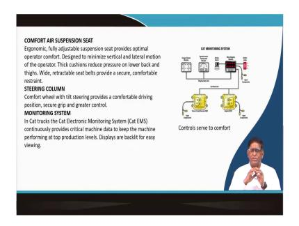
So, it is the comfort air suspension seat steering column and monitoring system all these are very well maintained. So, that means, the in a caterpillar trucks all the monitoring systems are done and it is controlled from the operator's cabin in such a way that while operator is easy to work and he gets warning for his safety as well as operational movement.
