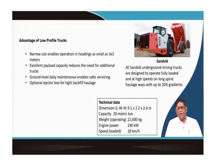
Now, why this low profile trucks are used that their main advantage is they are exactly narrow size enable operators in heading as small as 3 by 3 meters small gallery size they can work and they have got excellent payload capacity and reduces the need of additional truck is not needed here.
