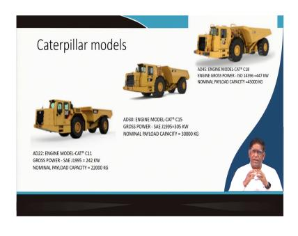
So, those are used in this. So, you can see this caterpillar models they have got this AD22, AD30 and AD45. These are depending on exactly on the capacity. These are the series basically, the technology wise they are more or less same only the selection of the engine and selection of the that size for the size; how the body is made?
