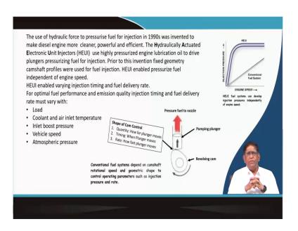
Now, the mechanically actuated that cam system is now removed over, here say as you can see normally what is there is a revolving cam is there which is connected to a cam follower and this ones will be this cam here this is driven taking the drive from the by a you can take by a bell drive or send drive or you can do a cam follower to drive with the from the crank shaft.
