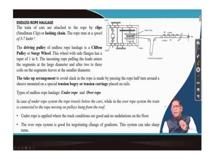
Then in this endless rope haulage a as you have seen this is basically a driving pulley which is called a Clifton pulley they do the operations and this can be done by two ways, it is under rope or over rope. In case of over rope in a gallery your rope is going at the top of the on the it is suspended from the roof and then the in a under rope it is laid on the floor.
