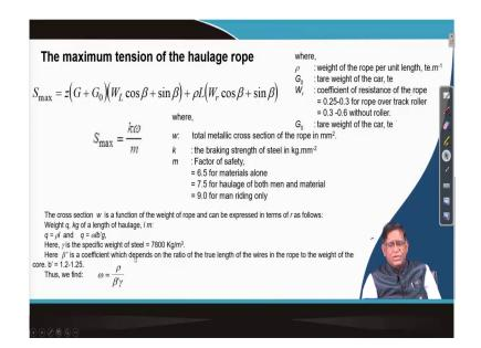
So, the maximum tension in the haulage rope you can find out the total load whatever is coming, that is your from the tear and the gross weight and then from the inclinations how much percentage of weight it is coming. And then what is the weight of the material gravity forces total is coming.
