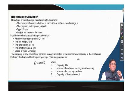
Now, coming to this the calculation is also very simple in these cases. Now what is there? We need to know that is how much is the driving power or how much is the capacity. So, this will be depending on the mainly the parameters which will be effecting, it is the haulage capacity will be effected by the net weight of that mine car. And then what is the tare weight that is exactly that is how much is the on the metals part of it and how much is the load part.
