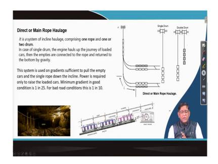
So, in the direct rope haulage is in which one drum and your things are being pulled, this is a single drum rope haulage this is a double drum rope haulage. And you can see here that is this is the roof of the gallery, you can see this is on the gallery you have got this the slipper and below that this ballast rocks are there, on that wooden slipper, on which this your, in a this here we are having the man riding cars.
