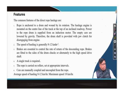
In your main features of a direct rope haulage is rope is anchored to the drum. Now, how the rope is anchored to the drum in a wire rope is that is called a coupling that is (Refer Time: 10:17) couple. That means, the rope one and is brought within the drum it gives a turning and there is a that is a group in which that your white metal is put over there to anchor it like that.
