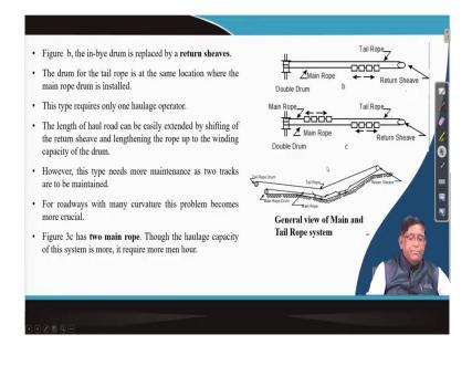
So, this here you can see here this is how these systems are working on the. The drum for the tail rope is at the same locations where the main rope drum is installed, by seeing the figure you can easily explain it. So, what it requires? Only one haulage operator because here this is only sheave.
