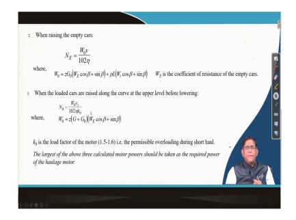
So that means, the motor power required for the empty drum or and that what is the motor power required for raising the loaded drum those things you can separately. And you can find out that what could be peak load during the operations of it.
