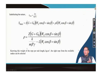
And by that once you determine these maximum tensions coming then you can find out what should be the density of the material of which that rope is made of. So, when you are going to buy wire rope for a haulage systems you must know that is what type of material that will have to be selected. If you do not do that there will be the problem of wire.
