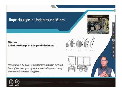
Now, today we will be discussing about this rope haulage as it was said in your previous class that in a rope haulage basically this is a tubs which are mine tubs you can see here this type of mine tubs which can be tilted that is here they are locked at this end. Now, this can be unlocked and it can dump the material from the side or there is a some such type of cars which can be one side of the wheels can be raised and then it can be it can be discharged sideways also.
