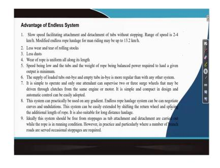
So, that endless rope haulage got advantages that it has slow speed facility. So, you can attach the tubs whenever it is there and the speed is normally 2 to 4 kilometer per hour. Whereas your in this can be with a change that is your by changing the gears and all you can run it up to 13.2 kilometer per hour also.
