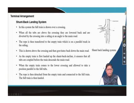
So, as you say as a terminal arrangement or the shunting back how they do. Suppose here you are having the haulage engines. These ropes which will be coming over here and the train will be brought up to here and then the empties will be brought on a shunting here, from here it will be that near the crossing they will be loaded to that. And then when that empty will be
