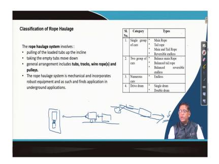
This a rope haulage system that can be classified into a single group of cars that is it will be main rope or tail rope, main and tail rope and reversible endless rope. And sometimes because this rope haulage system that cut that your rope all the mine cars they are exactly connected by these cars which are having on a wheel they will be travelling on this trail. Here you are having a coupling by which the next one will be connected.
