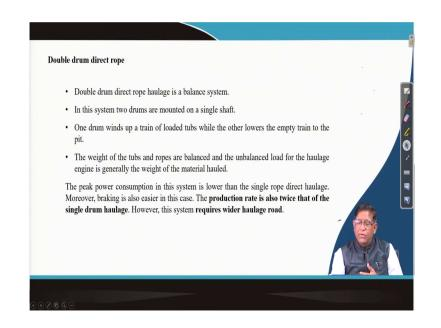
Now, in a double drum direct rope haulage there are two drums and they are mounted on the same shaft. So, one drum winds up that and then the other and other drum exactly takes the empty to down. Now, while this lower it is getting lowered that will be giving also some advantage. That means the motor will be requiring at least some amount of work is being done by the empty cars when they will be going down. So, that is why it is called a balance type of system because it is working withstand.
