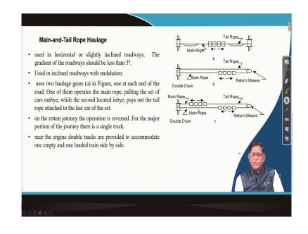
So, there is a other things other type of rope haulage, here you can see that there is a two drums. One that is your same rope exactly it can be while this drum will be pulling it up and this drum will be pulling it down. So, that is your that is your main and tail rope that is your tail side also a we are having a drive.
