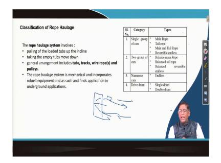
The same drum on a one particular drum we can have a two system can be maintained over there in between this will be there. Here this part will be having a rope in one directions, it will be releasing down here and this will be raising down here. So, that is you can go like that when your cars will be brought this will be emptied.
