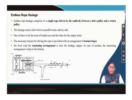
Now, the other thing in a next class I will be talking more about this endless rope haulage. In the endless rope haulage you are having the drive stations where a Clifton pulley or surge pulley is there. And this pulley with gear system is driven by a motor and then the rope is endless it is going over here and again it is turning at this.
