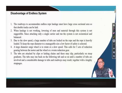
Now, but the disadvantage is the roadways to accommodate the endless rope haulage must be large cross sectional area. So, that double tracks can be laid. So, this is, in an endless rope haulage because the one end is taking another one is going down. So, as you have seen in that figure you need to make a wider gallery and then when haulage is not working lowering of man and material through this system is not suggestible.
