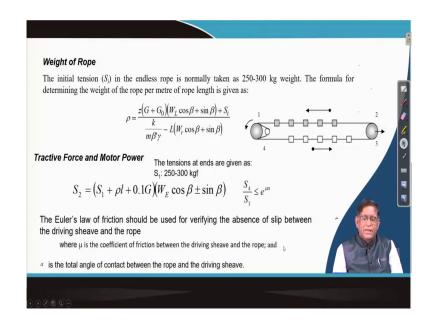
So, then how you select the weight that is your weight of the rope, that is your selection of this density as I said in the previous class that same way you can calculate out the tractive force and motor power by knowing how much will be the this your total load coming onto the system.
