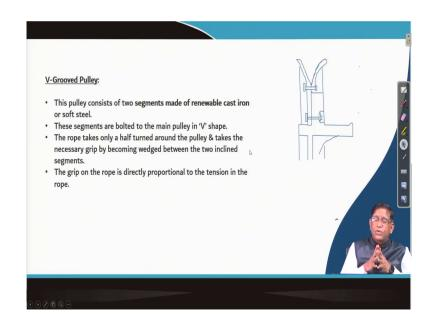
Similarly, a V-grooved pulley, a in a V-grooved pulley our there is a as the load is there that rope can be accommodated over here. So, this is a type of pulley which is used. And that there exactly two segments are there, and they are bolted together that is a bolted together and connected like this. So, that is the grip exactly if that more tension is there they will be just gripping it tightly. So, that is how a how it works.
