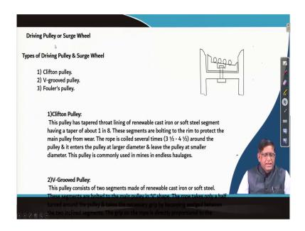
So, what exactly we have said that as you can see here there is a main called Clifton pulley. This is that most important thing for the drive this drive component can be of different types. There are called Clifton pulley, V-grooved pulley, and fouler pulley, that type of different type of pulleys are there.
