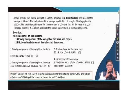
So, now I think you can do that whatever the basic principles you have learned on that you can take up a small numerical say a train of mine cars having a weight of 50 ton force is attached to a direct haulage. The speed of the haulage is 9 kilometer per hour given, and the inclination of the haulage road is given 1 in 10.
