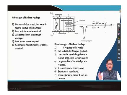
So, we have already discussed in our previous class that advantages and disadvantages of this endless rope haulage system is because of its low speed wear and tear is less. So, maintenance requirement is less, and a accident even if takes place sometimes their damages are not much, then your less motor power is required and a continuous flow of mineral or coal can be getting because all the time the rope is moving, so you are connecting.
