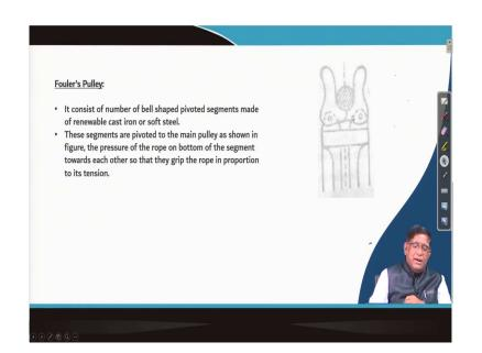
So, now there is a fouler pulley in which number of this is a bell shaped pulleys are there and they are just exactly connected to the that is your on your the main part you are just connecting this bell shaped one. Now, why it is a separable? If any wear and tear take place it will take place of the this portions, you take it out and connected another one and you can go on using.
