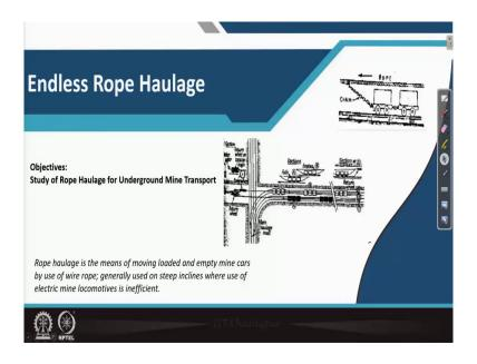
So, let us just go through quickly about what this endless rope haulage is. That one you have already you have studied that rope haulage. In any rope haulage, we are having a rope. Here we are showing an over rope, and in that rope our cars are connected with the help of a chain that is they are couple together, cars, mine cars are couple together running over this rails and then your chain by chain you are connecting it to the wire rope or by some clip or that lashing it is done.
