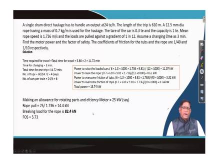
Another problem you can just say a single drum direct haulage has to handle an output of say 24 ton per hour. The length of the trip is 610 meter, 12.5 millimeter diameter rope having a mass of 0.7 kg per meter is used for the haulage. The tear of the wear car that is 0.3 ton, 0.3 ton weight car and the capacity is 1 ton. Mean rope speed is 1.736 meter per second, and the loads are pulled against the gradient of 1 in 12.
