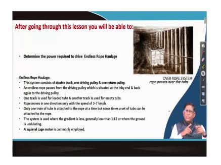
So, your in this system, we will be determining how the power required in a that is our main objectives today to do some calculations on the basis of this. So, this endless rope haulage it is a as we have already discussed it is consists of double track one driving pulley and one return pulley. So, if we somebody ask what are the main components? Very simple double track is required one driving pulley and one return pulley.
