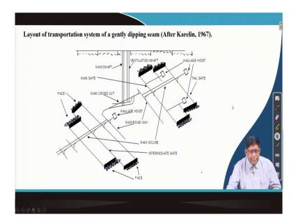
So, then, you can see here this another figure which can give you a total overall picture of the main layout, that is you can see here this is what we are telling as a main shaft. From the main shaft, it is coming and then, there is a main cross cut. It is a main gate, you can see here this is a haulage hoist is there; that means, a haulage hoist means a rope drum is there.
