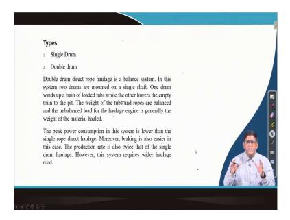
So, you will have to have a break arrangements and then, how on the track will be laid and what are the different safety devices will be there, that will have to study and then, as I have said already in the diagram. It could be by with one drum or double drum depending on that we can have a balanced or unbalanced systems.
