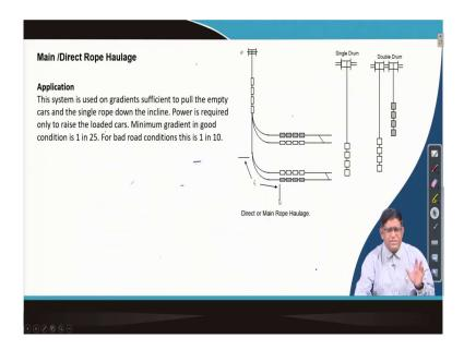
So, in a direct rope haulage, this one drum, it is carrying. This is a trait number of cars are drawn over here and this is way how a direct haulage work. This form a single drum, you are just carrying it up. If you put a double drum, your empties are going down and as your loaded are coming up or the vice versa, you can make arrangements with this.
