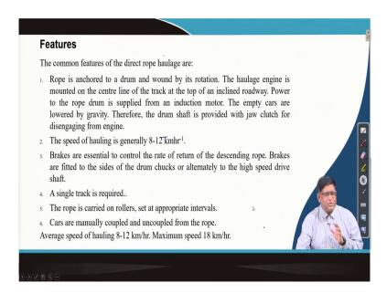
So, you will study about this main common features that is your how the rope will have to be anchored on a drum and the other side, it will be there with the cars. And that will be moving over a track and that speed will be about 8 to 12 kilometre per hour.
