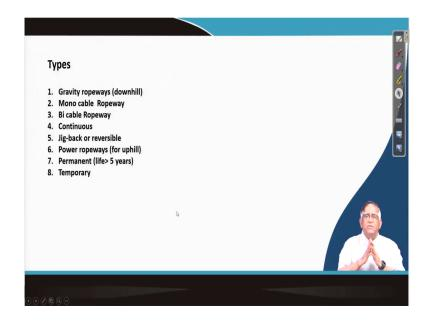
So, there are different types of this your rope way system. A gravity ropeways that is your mono cable bi cable it can be continuous ropeways jig back or reversible one will be going and then same rope will be coming like that that type of things, then there is a uphill. Uphill ropeway means you are exactly giving that power if it is a downhill ropeway then what will happen?
