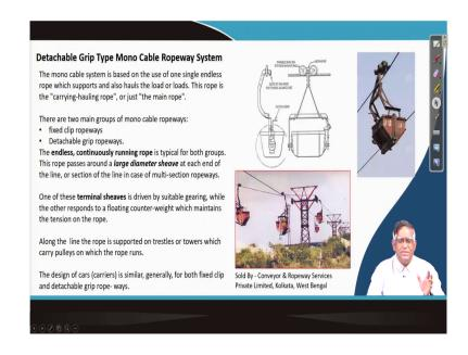
So, the other thing is we are telling about this monocable ropeway. In a monocable ropeway you can see that there is only one rope is there going over here on this rope you can see that this your that bucket or the container there is a your catch gear by which it is kept and then it has got the wheelchair wire which is having a grip.
