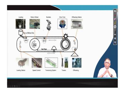
So, basically what that aerial rope way system is, that you are having a continuous endless rope is running over here, this is called your haul rope and then there you are connecting these buckets.
