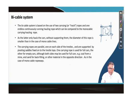
Now, if you see that in a bi cable system there are of course, the 2 cables. Now on that 2 cable there are systems sometimes you have got the 2 cables like that and you may have a 2 cables on this even a trolley like this we can have on a 4 wheels it can go over here the material will be loaded in this bucket.
