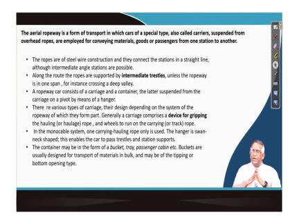
Now, the aerial ropeway is a form of transport in which is as a special type, also it is called a carrier that or somebody say it is a car or a tub whatever it is there, it is suspended from the overhead ropes and they are exactly can be filled you will have to how you will be loading the material.
