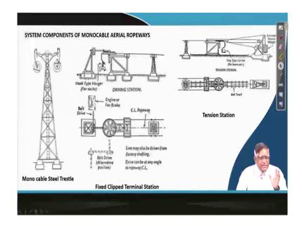
If you see here this is a trestle on which this rope will be going one for you are going say towards the from the upward and the another is going downward or one is for carrying side, one is for your return side. This is the loaded one will be going from here and you can see that empty that is a reversed one it is coming this way.
