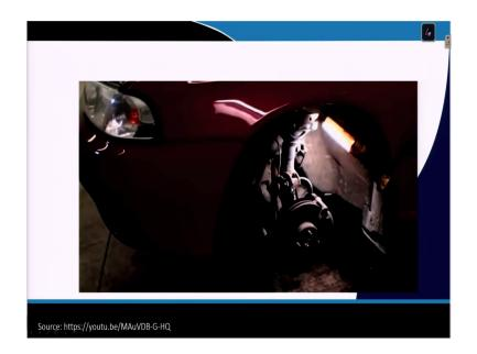
And you can see that in any car, if you open up the that take out the wheel; you can see this is that on that your this axial how this block; here we are having this brake shoes are over here. Now, we can see that in a wheel the mainly there is a that, your main brake caliper assembly, this is fitted over here and outside that disc brake that part is there and then the wheel hub assembly.
