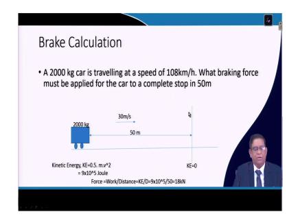
But here you can do one small calculations; if you are having a 2000 kg car is travelling at a speed of say 108 kilometer per hour; what braking force must be applied to that car to be complete stop at 50 meter? So, if it is coming over there, within this 50 meter it will have to serve. So, what is the basic principle?
