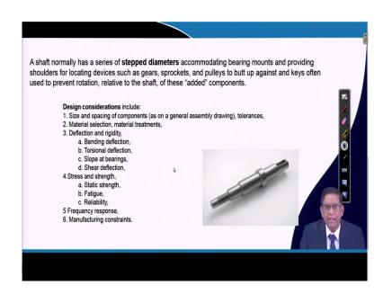
Now, they have, as you can see here; this is a picture photograph of a shaft which is used. So, it is normally you can find like that a stepped diameters are there. So, and there on these you will be mounting the gears, sprockets or pulleys, so that the different purposes in the machines can be done.
