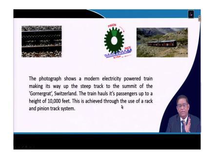
So, like that, you have got the different types of gear used in a of this; as we are seeing here, this is a rack and pinion systems. This it is it in Switzerland there is a place called Gornergrat; there the railway lines are because it is in a very steep slope, the train moves and for that the whole drive systems, it is exactly they are having a rack and pinion type of arrangements over there.
