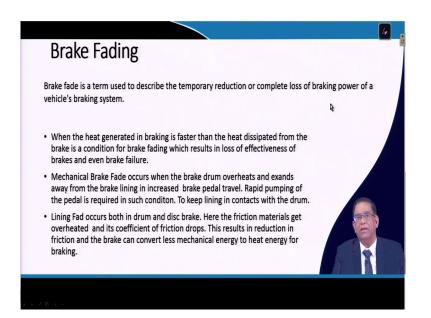
And then what happens in any brake, whether the brake shoe is there on the drum; then because of the frictions over there, there will be always wear and tear, that at that time that phenomena is called your brake fading, where exactly the temporary reduction of the complete loss of braking. If the brake is fading, then your there will be a that is it will take the longer distance to stop or sometimes it may not stop and which may lead to accident. So, that need to be system.
