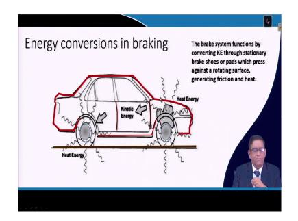
So, these brakes are very important component; you can see what is happening in a energy conversion takes place in a brake. So, when a car is moving, when this is having a lot of kinetic energy; then you apply the brake, then this kinetic energy is dissipated as a heat energy and then ultimately you are stopping the car.
