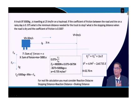
So, some such type of problems you can do; even sometimes a problem can be say, if you are having a truck with 5000 kg is travelling at a 25 kilometer per hour on a haulroad. If the coefficient of friction between the road and the tire is given, it is 0.75; then what will be the minimum distance?
