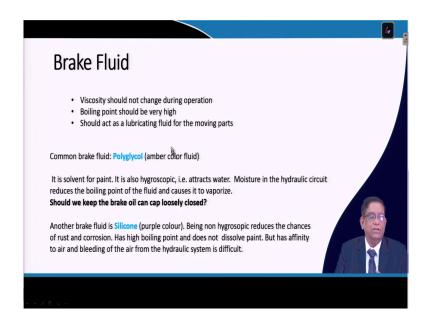
Now, this brake fluids normally the polyglycol or silicone fluids are used; but one need to be very careful about selecting this brake fluid, its a it should not be at contaminated with water, because that water will be deteriorating the things.
