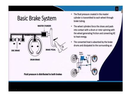
So, these arrangements of breaking in a normal car you are having. But what exactly the brake system work; if you are giving a brake pedal at that time, there is a master cylinder, from the master cylinder that fluid brake oil is distributed; either it is going to the front and the rear side. As you can see over here, there is by pedaling over here; from the master cylinder fluids are going and then they get distributed to the their front wheel and the rear wheel.
