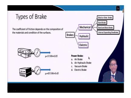
So, this there are different types of brakes exactly; you know that whole braking system it is a matter of principle is there friction. As you know that this here that coefficient of friction, that is exactly if you are taking a ice slab and then if you are pulling that thing to that on a rubber pad; if your ice slab is there, it will be just by giving only five that unit of your force is giving.
