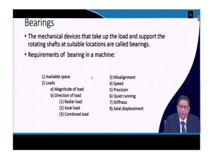
So, this pulleys are, this type of sheaves are that; the next important things you will be knowing about in the mining machinery is the bearings. Most of the machines they sometimes under brake down, because of the problem with bearings. If the say for example, in a drilling machines, when your drill bit is cutting at a depth; at that time a lot of heat is generated and also there is a your the bit is rotating against a bearing.
