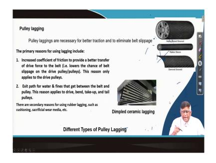
Then the pulley lagging I said so that the your slip does not occur for that on the drum you will have to put this type of lagging, and sometime dump ceramic laggings are also put over there. So, that the frictions that e to the power mu that that mu part is kept more.
