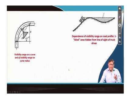
So, this is the way how we can derive these equations and calculate we need to do it. Because while doing it, you will have to see that what is the safe distance that will have to be there in the mine. If a this type of situations comes so that there will not be a vision that is a you cannot see the other truck, if it is coming over here.
