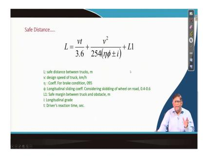
So, this is the way you can calculate this. Similarly, that what should be the safe distance between two trucks and then, what should be when you are brake at that time, where it should stop. So, that can be calculated from the equipment that is your you will have to maintain this safe distance between trucks, depending on your design speed.
