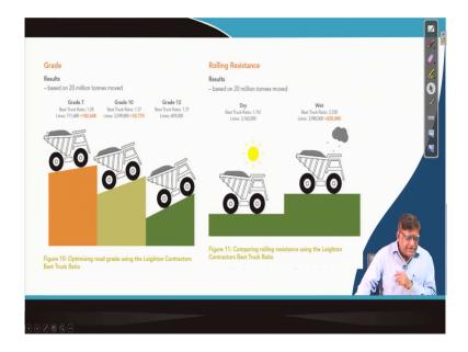
Similarly, this can be for that your how in the grade, it is working in this gradient you are working at this gradient working in these gradient. So, the gradient wise, your best truck ratio you are given when the grade 7 is there, in that you got the best truck ratio here 1 is to 7. Similarly, under the different conditions that is your in a rainy season or in a cloudy season, depending on that also you see that finding out the best truck ratio, you can identify where it will work.
