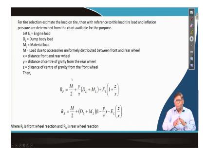
Similarly, another things you must know that a truck overall truck load that will be that is how much reactions will be coming in the front wheel and the rear wheel. These will be depending on the total load and that accessories which is coming over here and the distance between the front and rear wheel, that is the what is the length curve.
