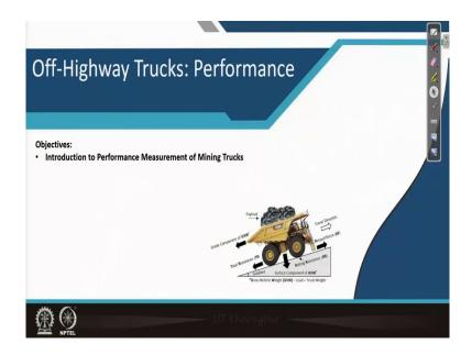
So, this particular class is for introduction to the performance measurement of mining trucks. This is a as we know that is our main job. Here we have discussed the truck will be deployed for carrying material from the pit to the surface. So, it will be going with a payload on it up a gradient and then, it will have to overcome different resistances.
