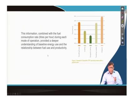
So, that is your how much time the truck is operating with which mode say that means, travelling empty, loading that you are stopped during for loading, travelling loaded and stop loaded, these conditions how much time, it has taken. This overall scenario will be affecting the total performance and energy consumptions.
