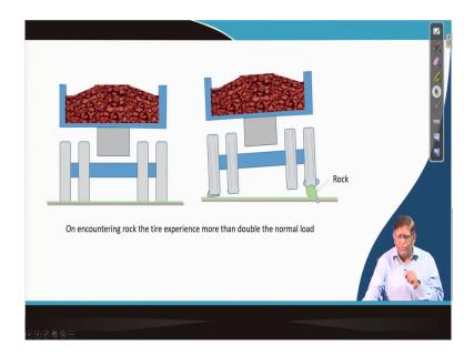
So, this way when you determine, this that normal reactions which come, it is important because the total load which is coming, it should get distributed to all tires equally. If now on the road a rock comes over here, then what will happen? The whole load will be coming onto one tire that will be getting over and this tire will get damaged and it will be loss.
