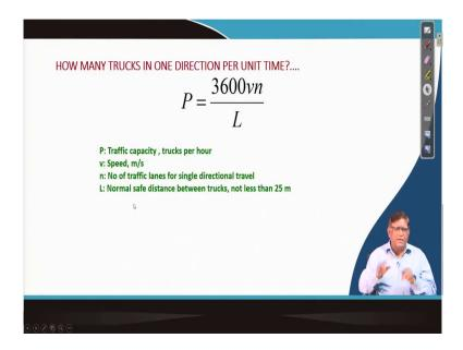
So, that is why the whole overall your road infrastructures which have been developed in the mines that will also affect. So, this way some performance-based standards are determined. Other things which you need to know is how many trucks in one direction per unit time. You can calculate it from the speed and the number of traffic lengths which you are having and the normal shape distance between trucks, how will you have to find.
