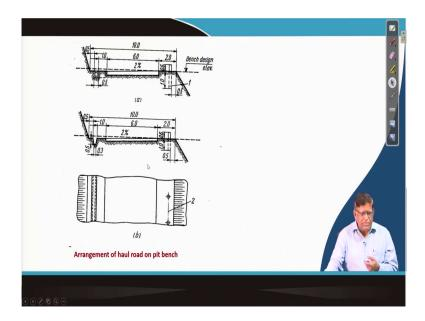
So, that means, the haul roads design that is whether there will be a proper gradient, there will be safety bomb and this you do in surface mining, when you do a haul road design. So, that means, for the performance of the truck, these two things should be comfortable that how will be deploying the truck on a things.
