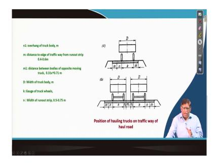
So, then you will have to see that truck, how it will be exactly maintaining your the truck body on a haul road, when it will be making how that two trucks will be having at how much distance. All these things are as a normal standard procedure are given; you will have to put; then, only you can achieve the proper performance of the truck.
