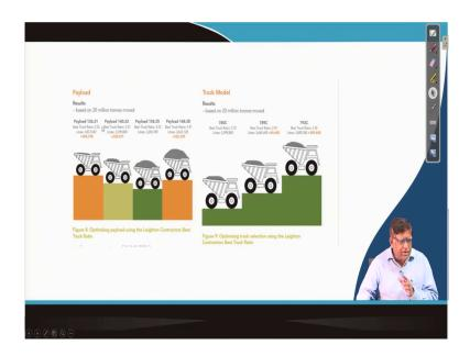
Now, these best truck ratio, when you compare you can see here that is your your best truck ratio is a 2.55 for a payload of 126.21 tonne for a particular truck. In a case study, people have studied like this and you can see that the best truck ratio that with a payload even less. So, that means, that by just only having a higher truck itself will not give you the best performance.
