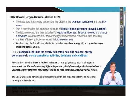
So, that is why that this new methodology that downer energy and emissions measures, they take the total fuel consumed and total bench cubic meter transported that they convert this into how many liters of diesel per tonne moved. So, from cubic meter, they take it to the per
