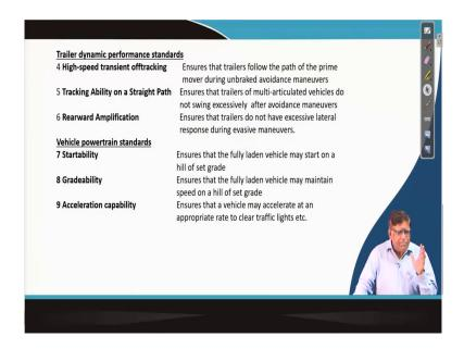
So, there will be trailer dynamic performance standards. Sometimes you use articulated truck. When you are using articulated truck, that the trailer which you are connecting. So, they will have to take certain measurement. So, your high speed transient off tracking that is your trailers follow the part of the prime mover, that is your that main that engine and that which is prime mover which is taking the trailer away, they will have to follow the same alignment and do while we are doing.
