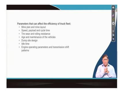
So, basically, this is a you will have to take care of what are the different parameters that will be affecting the efficiency of the truck. The efficiency of this truck will be as a it will be truck will be always working in a fleet. Because to serve 1 shovel, you may have to have depending on your side configurations 4 trucks, 5 trucks, 7 trucks depending on the situations how that it planned it.
