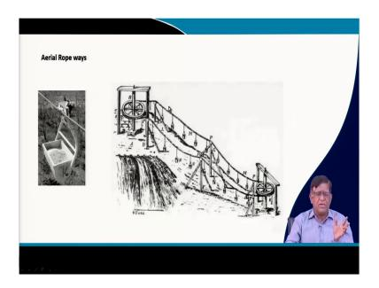
So, you can see this rope con and then, you can study. Then, there is a aerial ropeway which is a one of the very old system, still it has got lot of potential for using many of the places; but because of its low capacity, because of its intermittent nature, it has not been used.
