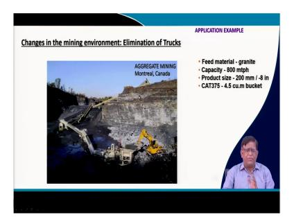
So, you can see here that is a without truck, there is no truck, so no maintenance of haul road, you can just do a query operations by this. There is also this is a metro a companies, they have given a this type of mobile conveyor system. There is a conveyor belt over here, which is mounted on these tire mounted systems on which it can move, it can make number of them combining together and taking out of the pit.
