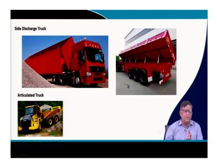
This one you can see as a side discharge truck; the truck is having that is your the hydraulic pistons are working from the side, unlike that rear discharge, it is a discharging at a side. Sometimes, this can be depending on the where you are loading, you can have. So, these are the innovations people have done wherever it is there.
