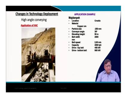
But there, this conveyor belt normally the conveyor belt cannot go more than that is a angle of repose. Because if a conveyor belt you have took the material, if the material angle of reposes, its normally it will slide down with that. If the angle of inclination of the conveyor belt is more than this, this angle, if it is more than the angle of repose, then the material will slide down.
