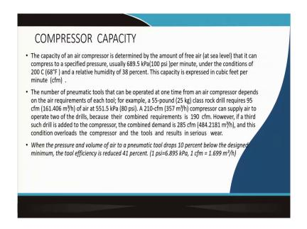
So, now you have basically learnt type wise, you have got number of different types the primarily you are reciprocating types, that your rotary type, that is particularly the screw compressors and also axial flow compressor these are the used in our industry. Now, one most important thing to know about that what is the capacity of the compressor. The capacity of the compressors is exactly that how much free air that can be compressed and then to a specified pressure.
