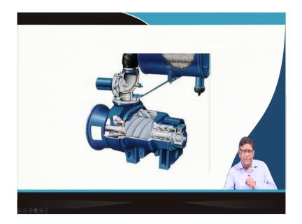
So, if you see a single stage that how within a casing, how the screws are put over there and then from their how from the intake air will be going out that you can see here there is a air filter at the top, you can see the air is sucked through this filter. So, that it is coming over here and it is going out at this end. So, by that the all the dust particles and others are removed or kept away from the compressor.
