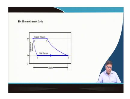
One basic things of the thermodynamic cycle should be clear to you, as I was telling in the reciprocating compressors in the three pistons, then when you are just bringing the piston down at a lower point at that time this much volume is sucked. So, this is a volume and this is your pressure, the pressure volume diagram, it gives that exactly how the thermodynamic behavior of the compressors.
