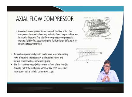
Other book which I referred to you as a pump fan and compressor that books gives the detail of it of the theory. The other that is your reciprocating and then screw type your centrifugal type you have seen there is another type of compressor switch is called axial flow compressor. In an axial flow means the flow is inner the in a parallel to that shafts.
