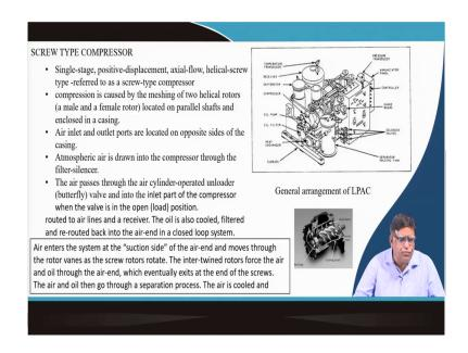
So, that means depending on how you use these compressors can be different. So, if you talk of a screw type compressors, here in this diagram you can see a there are two screws- one is exactly called male rotor and there is a female that is your rotor.
