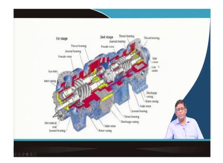
So, this is a there must be a cooling system and then there must be because that cooling system sometimes with the oil also. You can see in this figure, there is a how there are 2 stage- this is a 1st stage and there is a 2nd stage; that means, whatever will be pressurized, that pressurized air is getting further pressurized and it will be there.
