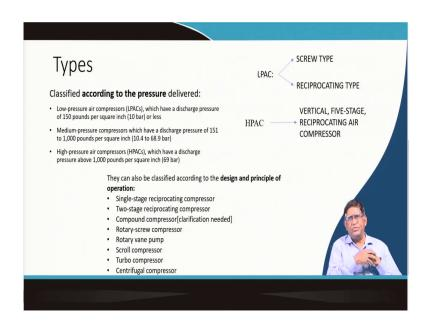
So, this compressors, we need to know that there are different types of compressors are there; depending on what is there exactly your low pressure air compressors, which the pressure range will be within 10 bar that is a low pressure. Sometimes it can go up to say 70 bar 60 that is 10 to 70 bar that is your up to 1000 PSI that is around 68.9 bar, that is a medium range of air compressors, then there are also some higher size air compressors where this is pressures they can generate much more.
