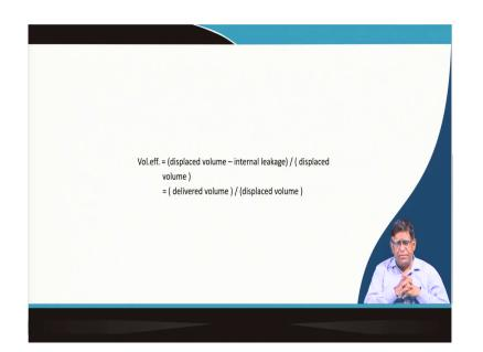
Now, the volume efficiency of a compressor is determined by what is the displaced volume and what is the internal leakage and then divide by the displaced volume. So, that is what exactly your delivered volume by the displaced volume, that gives the volumetric efficiency. So, you can easily find out from the rating and then you can find out while we are operating, if there is a volumetric efficiency is reducing, that you need to take proper actions that how you can improve it.
