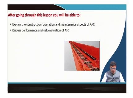
You can see that those pans, they join together and then they make a total chain conveyor over here. So, now we will be discussing about this chain conveyor, how they are working in front of a along with a shearer and power supports.
