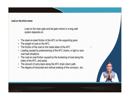
So, now the main thing over that how much load on the main gate and tail gate motors and that in that system will be coming that will be depending on that how the what are the different resistances. So, that means, to drive the chain and the conveyor material over there, your the how to decide that what will be the motor power required to drive it that load will be different resistances.
