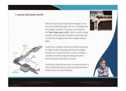
Now, that all the pan that you can see that if this is your the main chain conveyor that armoured face conveyor, your shearer is here, these pans are connected together to form it. You can see this is the that shield or the support system, power support is there.
