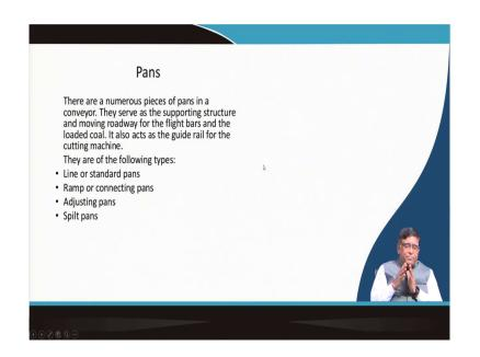
Now, these pans which are exactly coming in a number of them, they will be joining together by that your a pins and then, that is why there are different types of pans are available, it can be a line or standard pans, ramp or connecting pans and adjusting pan and split pans.
