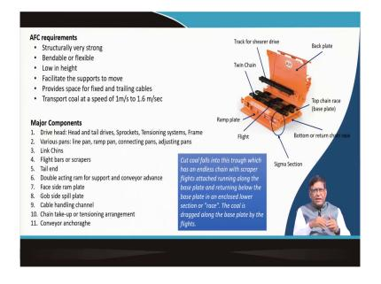
Now, let us little bit of more detail, you can know about what are its requirements. If that is to work in a longwall coal mining which can produce you can you might have heard that there is a with the shearer, when I talked about this I curves 1000 that is which can give up to 6, the up to 1 to 6 million ton of coal can be produced from 1 longwall mining that is say longwall mining is a high producing mine.
