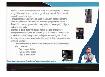
As you see, this is a AFC, it is exactly made up of some short sections. Now, this small short sections are called pans. As you have seen in the previous diagram that it is coming as a this is one pan. Now, like that it is made up of this pans and then, it allows to snake along or that is the it is as the supports and the progressively advanced.
