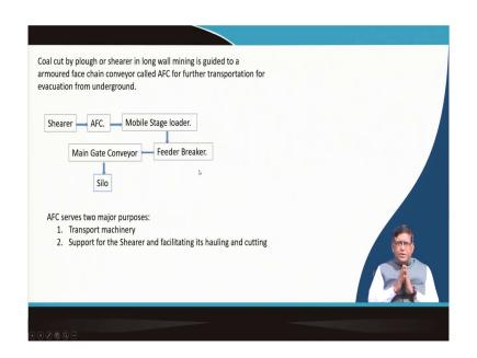
So, if we see that how exactly the coal is a taken out by longwall mining, we know that our plough or shearer these two are the main machines which are used for cutting the coal from the seam.
