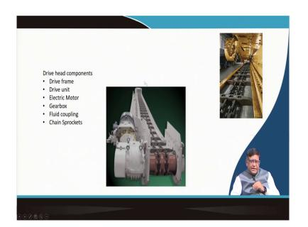
Now, you can see here that is this is the your end drive, you have seen the motor and then the couplers, then we are having this sprockets and this shaft is being driven. So, this is the drive head part of it where you are having this frame, drive unit, motor, fluid coupling and the chains sprockets.
