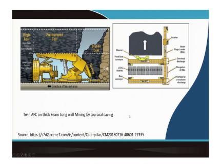
But the another thing is very important that is so far we have said that this coal seam is a very thin seams there we are working. Now, there is a method in longwall mining called your top coal caving. Now, that means here you cut to certain extents, then the upper portion of the thick coal seam are allowed to cave in and then caved one also will have to be carried out.
