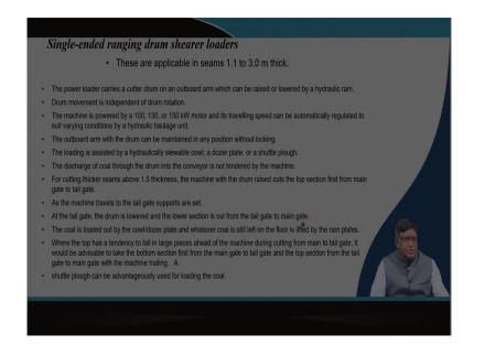
So, there is a that the single ended ranging drum shearer which can be used for single ended means if you are having only one drum, it will be cutting like that. Now, if you are having two drums, one cutting from here, another cutting over there that means, the total thickness can be managed. If you kept two drums position like this that means, from here to here, this part of the your coal face can be cut.
