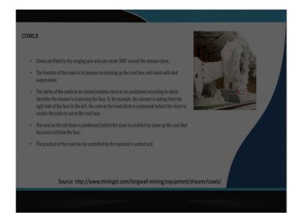
So, as such for this purposes, your these machines component wise you need to know. As I was telling that one major component is that cowl that means, when this shearer will be rotating like that, it will be cutting say if it is rotating in this directions from the bottom to top it is moving, then this material will get guided over here so, this vane and that this cowl will be guiding it to the that your armour face conveyors.
