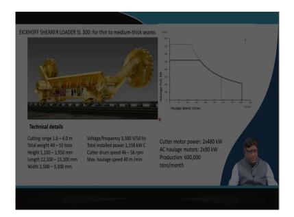
So, if you see that is there to get the high production rate that is a different way it got developed say I am telling as an example Eickhoff SL 300 and this SL 300, then came SL 500 then came SL 750, SL 1000 big machines. You can see there, how much haulage pull is there and how much haulage speed is there. This curve that exactly shows that how much kilo Newton haulage pull can work with that, what is that velocity?
