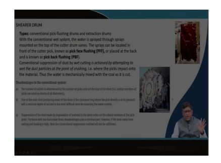
So, I hope now you have understood that what is this machines constructionally. Then, you may go on studying the type of drums which can be there. There are different types of drum depending on how the flushing or how that water spraying is done that is why they have got two types; one is your pick face flushing and pick back flushing.
