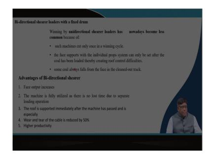
So, that is your the bi-directionals, when you make that cutting in while both the directions you will be cutting, that has got that advantage because it can give a more output because total overall cutting time is more ok. So, then if you are that main importance of the bi-directional shearer is you are fully utilizing the available time.
