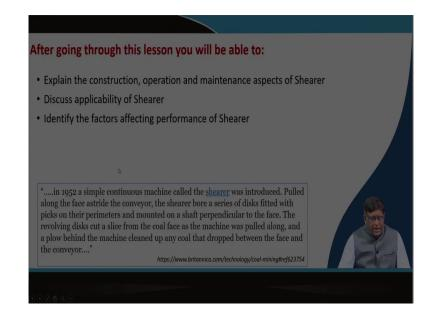
So, this lecture is mean for that after that you should be able to explain how these machines work exactly, what are their the constructions, today we will be introducing about the shearer, in our subsequent classes we will discuss about armour face conveyor that is a flexible conveyor and also we will discuss power supports and in general, we will be discussing in our future class about how these machines are exactly maintained.
