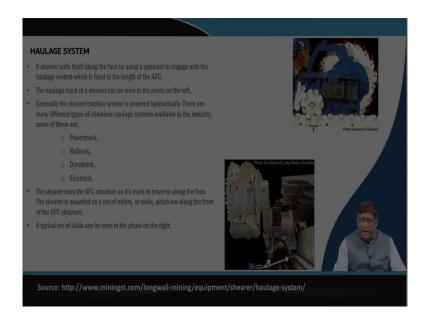
So, then the haulage of this that how this machine moves exactly you can see a trucks can be kept on the that your the armour face conveyor on the AFC, it can be as a rake and pinion or it can be a chain on which a sprocket will be moving that this that pinion or the sprocket is a mounted on the machine and then, when it will be rotating then as it is a fixed rake or a chain that machines will moving.
