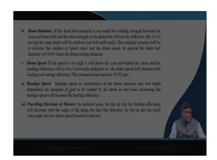
And then, you can find out that how you can do that your loading efficiency you can improve by that factors like your helix angle, by your vane spacing, vane depth, drum diameter, drum speed, haulage speed, traveling directions.
