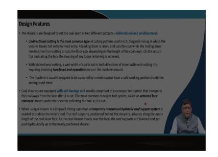
So, that main design features is whether it will be your unidirectional or two-directionals and whether it has got your a automated self-haulage unit or you have got a separately from outside, you need to give that chain can be moved separately and then, the machines will be moving. So, there could be a different haulage systems there.
