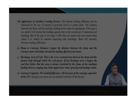
Then, your auxiliary loading devices which you are having, then your what is the distance between the drum to the conveyor, how that exactly discharge of that discharge area for that coal, your conveyor capacity all those parameters need to be studied.
