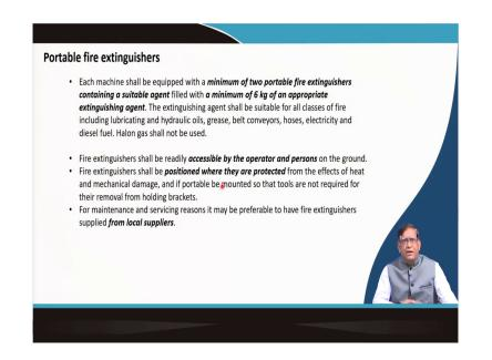
Like that you have got the, you can keep some portable fire extinguishers also in the face, so that in any case if the machines any part gets any flame, it can be put.
