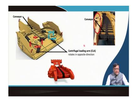
So, if you see here as a constructional component wise that, this part you which you have seen here; that is in your the gathering part, here it is exactly we are having two centrifugal loading arm is there. You can see that they are rotating in the opposite direction, this is rotating in this directions and then this is rotating in this directions by which the material are brought over here in front.
