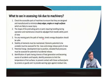
Now, what most important thing is you need to work with this machines in underground. When you are working with any machines in an underground coal mining, you need to be very careful about that to avoid accidents and then avoid mishaps.
