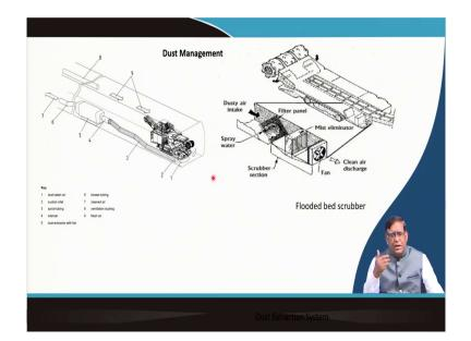
So, that is what exactly in a machines, most important thing is that dust management. You can see here these two type of dust management over there, that is your the from the dust, flood, and air when it is coming from the front of it; it is going through the suction inlet and then it is going to the spiral that you are tubing, then it goes to a silencers and then it is going to a dust extraction fan.
