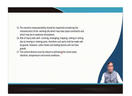
So, this is general thing which you must know while ever working with any underground machinery. Moreover the maneuverability, sometimes this machine will have to be positioned for maintenance; it will have to just see that adjust for the if any side wall fall or anything takes place. So, that is why the maneuverability of the machine, so that you can steer properly within that limited space need to be seen.
