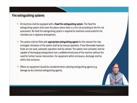
So, and so after ascertaining that, you will have to develop and give some fire extinguishing system, that could be a fixed type of fire extinguishing system. But and that what type of agent you use; that is whether for electrical fire or for the gas fire, you will have to get the fire extinguisher with the proper fire extinguishing as it should be there in the machines.
