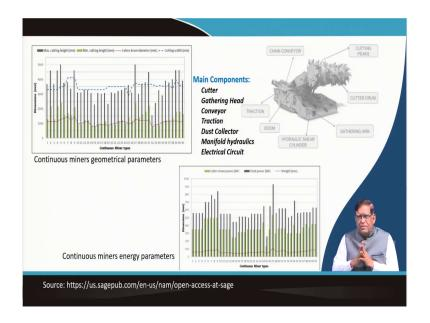
So, if you see that to say there is a quite a good number of machines from different manufacturers are available; but structurally if you see, it is comprising of some basic components. That components main is that your a cutter head, that is the cutting the main rock cutting is done by the cutter, where which is having certain cutting peaks or as you can see in this figure, that peaks are on a peak box mounted on the scrolls.
