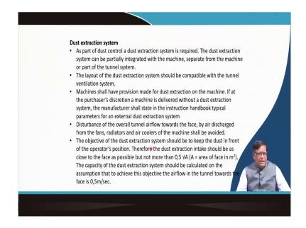
Similarly, the dust extraction system is very very important; because as I said this coal mining dust is can it can generate pneumoconiosis amongst the miner. So, for the dust collections, we
