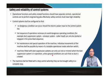
So, the safety and reliability of the control systems, exactly it is you will have to see that there is no dangerous conditions can occur. And sequence of operations in which way it will start and which it will a it will have to be close; to shutting down and starting sequences as prescribed by the your operators manual need to be maintained.
