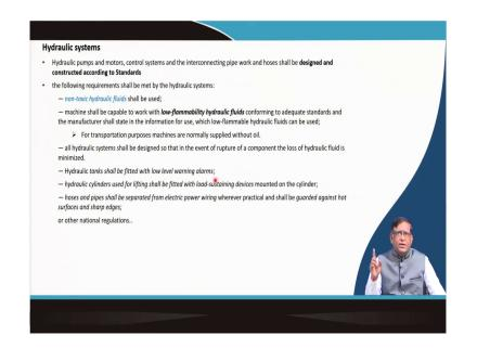
Similarly, the machines you have got a lot of hydraulic systems, because there are that is your hydraulically controlled that is your motor as well as different actuators are there. So, for that the fluid, it should not be a toxic type or an inflammable type; then the pressure generated, it should be that your all the host pipes should be with the proper specification, so that the under operating pressures and temperature no leak generates and it will be there.
