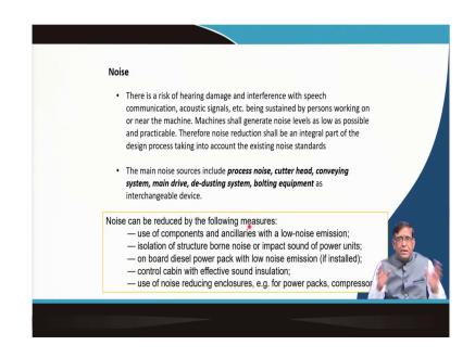
So, will be another problem is this noise, because it is a mechanical loosening of coal, while cutting that the overcoming this cutting resistance. The basic principle of shearing, where there will be a lot of noise generated; moreover the machines also can vibrate, because of the machines different parts vibrating, a lot of noise will be coming.
