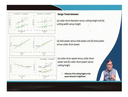
Now, there is a if you see the design trends of this machine, it also shows that this cutter drum diameter; if you see that your this and then cutting height, if you see the cutting height and drum diameter, as your drum diameter increases, the cutting height increases.
