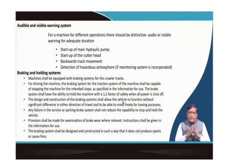
So, then your there will be the warning systems. So, particularly in this machine, the warnings are given for the startup for the main hydraulic pump is working or not startup of the cutter head; then your backward or track movement, if you are moving in a reverse motion or if you see any dangerous situations coming in all these cases, there should be a sufficient warning that could be a audible or a visible warning could be provided.
