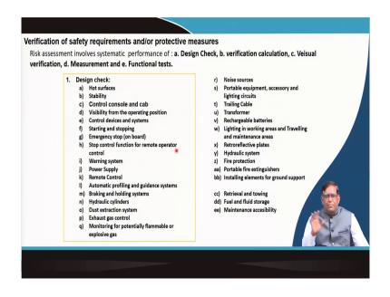
So, whenever you go that the protective measures, there are number of checks need to be there. So, whenever you are going to inspect this machines, make a checklist for that what are the design checks will be doing; like that whether the hot surfaces stability, all the points which I have just said are listed over there. You please make this list and so that you can make a have a point; that if you are going underground to inspect a machines, what are the things to be looked into.
