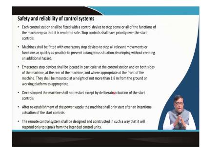
So, this the control stations should be there in the machines from where all the operations can be monitored; then it must be fitted with the emergency stop. As I said that is if you see that something is wrong, some fall is coming up, there you are apprehending that the machine may get jam or stuck or it can get unstable; at that time, there should be a button from which exactly emergency stop you can operate with, ok.
