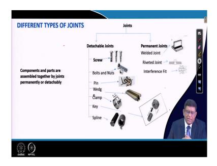
So, now while constructing the machine you will be finding that there will be different type of connections are there different parts will have to be connected together. Now, there comes these joints and while connecting or jointing these two different parts there can be a permanent joint or there can be a detachable joint. In the permanent joints you might have already heard and seen many places that the welding joints are there that is to permanently you are joining by welding.
