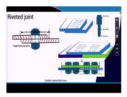
So, these different joints are there. Now, what is a riveted joint? A rivet is a small piece of item that is like that is has got a rivet head, a rivet shank and rivet tail. Now, two plates are there that is if this is to be join together that what they do? Just put this a your rivet inside and then you connect the tap shielding it over there you join it.
