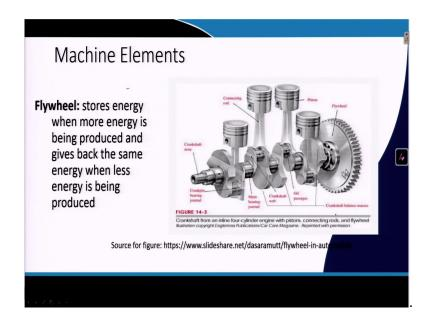
When the shaft around that the lubricant oil will be there how this type of different types of bearing how it works you need to study for this. So, that what is the purpose of this flywheel? Because this machines at different time there will be fluctuations of its emotions and all, but here from with flywheel thus power will be taken to a your transmission system and from that transmission system when it will be going to the main drive.
