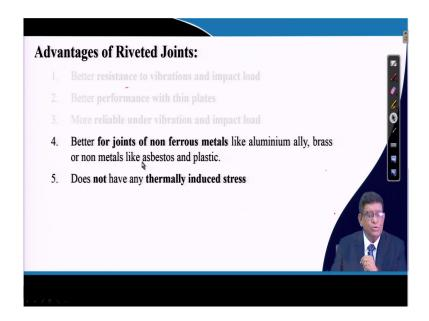
They are having also better for joints of nonferrous metals. So, does not have any thermally induced stress exactly we will find we will talk about that when you do welding it is exactly lot of thermally induced stresses are there.
