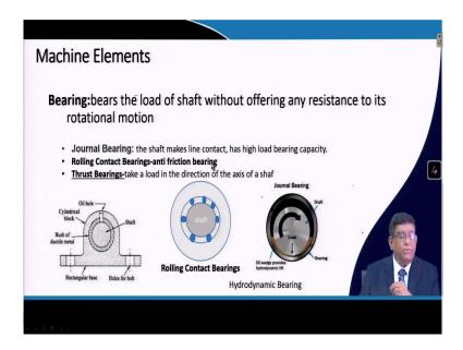
And then we have got in some cases the bearing is another part when it is a shaft is to rotate it is say there will be the frictional loss will have to be minimum. So, that is why different of bearings are there that is exactly how a shaft is mounted that is it can be a general bearing, it can be a rolling contact bearing or it can be a hydrodynamic bearing.
