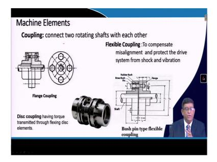
So, then other thing is there in a machines you will be having the coupling when your two rotating shaft a which are at motion if that we given a connections they called a coupling.
