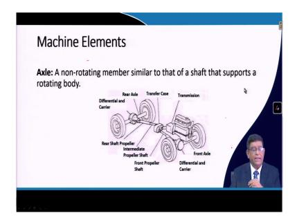
So, that you can see in the machine elements like in a car how the power is going from one end to another, you can see that these wheels are having an axial we have got a propeller shafts then we have got exactly intermediate propeller shafts can be there and then we have got the front axle that your a differential carrier. So, that again a power transmission system such type of elements are made together to work with that.
