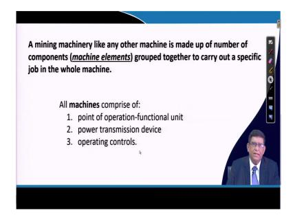
So, for that you know that mining machinery like any other machines is made of this component which we are calling it as a machine element. Now, the machine exactly it is made up of some point of operation or functional units. So, that is say any machine see even if you talk of your sewing machine, in that what is there? There is a point of operation is the needle which is moving up and down and that is the main functional unit.
