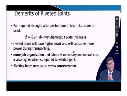
Exactly, when you make a riveted joints you were making a lot of holes in a main parts. So, that way it is the parts get damaged; moreover as you have seen whether it is a lap joint or butt joint that you use an extra plate over there. So, when you put an extra plate; that means, you are going to increase the weight of the machine. And if any machinery which is a moving
