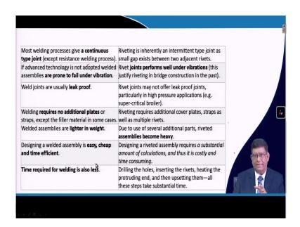
So, you can see that there are a you can get a continuous type of joint in case of welding, but in case of rivet as because you are having these holes and then that you are putting the rivet it is not a continuous one. So, that is why the welded joint will be leak proof, but riveted joint
