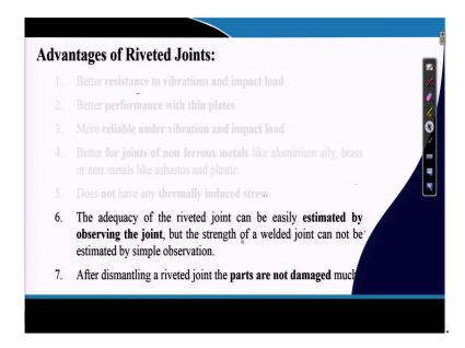
So, the adequacy of the riveted joint can be easily estimated by observing the joints. You can see the joint and by seeing that you can know that whether it is exactly or not, but in a welded joint some time there could be inside it could be very weak or it can be having some problem we do not know and then the by just simply the inspecting you may not be able to find out that a particular joint has become very weak.
