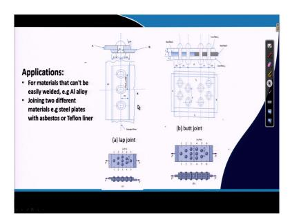
So, you can see here that the riveted lap joint and butt joints they can do that can be done the butt joint can be done giving two plates one at the top one at a bottom by that way. So, there could be a different type of requirements depending on the type of strength it is required you may have different type of riveted joints like your lap joint or butt joints.
