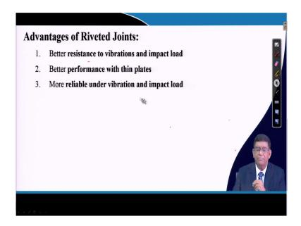
So, these riveted joints are better resistance to vibrations and impact load, better performance with thin plates, more reliable under vibration and impact load.
