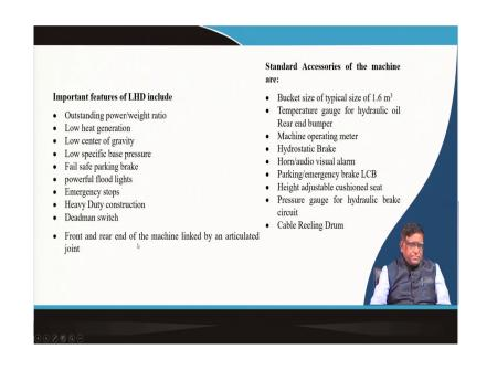
So, there are many features are there particularly, it is an outstanding power to weight ratio, whenever you are going to select a machines this is a parameter you need to find out that is it is a what is the install power and what is the total weight that ratio exactly has an impact on your operating cost.
