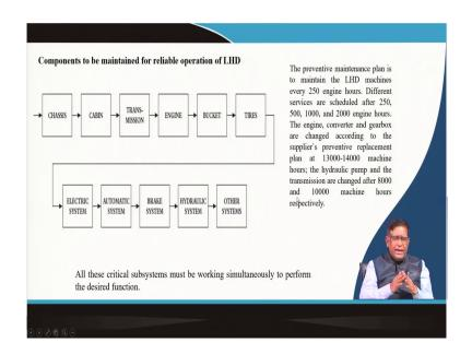
But you will be knowing that the component wise, in the machines has got the chassis, cabin, transmission, engine, bucket, then tires, then electrical system, automatic system, brake system, hydraulic system and other system. So, each of the systems reliability you can study that could be another innovative work you can do it over there, how exactly you can store the data, you will have to have.
