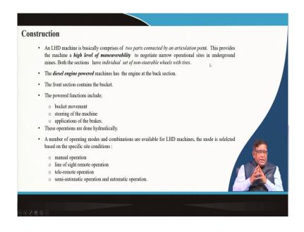
So, now coming to the construction wise, you have seen the photograph here of this machine. So, this is basically it has got this two parts, the front part and the rear part, they are connected at an articulation point so that this, the there is a good maneuverability because if the front part is connected and in between so, keeping one fixed, the other can take a turn and or distance keeping this is there, it can get a turn.
