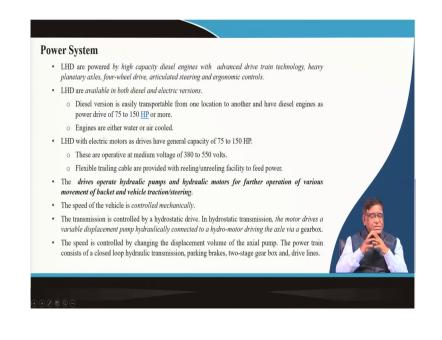
Now, it can its capacity as it is there that depending on the size of the machine, size of the gallery, there could be a different size of the bucket and then, they can work. But the power system as you can see here, it is by high capacity diesel engine or by electrical, it is available in both the versions that engine capacity it can go up to 150 HP.
