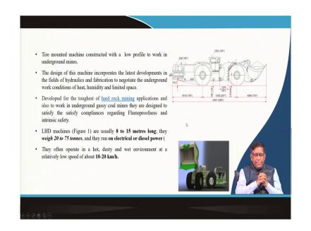
So, you can see here as the machine, when it is said an articulated, you have got this as a front part and this is rear part, these two part they get connected with a that is your, so that we can easily move around and then take a turn with this. So, this machine can be a tire mounted machine and it is exactly work, it is a design to work at a low profile that center of gravity is long below and there is a good stability of this machine.
