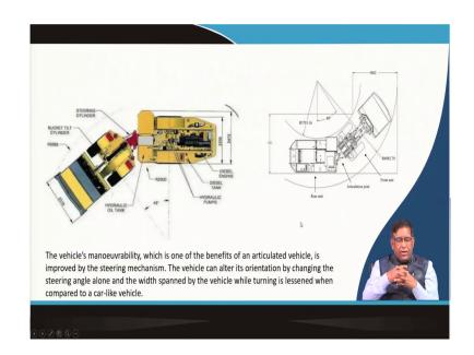
Now, you can see here the manoeuvrability that is to negotiating in the curve always is possible because of these articulations. There is a steering cylinder by putting pushing this out, you can make the things exactly keeping this one fix, you can take a turnover here.
