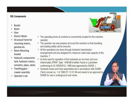
So, you can now summarize that what are the main components which will be there in any machines. So, whenever you have been studying, you know that there will be the bucket and then the bucket will be supported on a boom; then the boom will be supported on the super that is your the chassis or that, then this will be on a structures which will be having the under carries unit.
