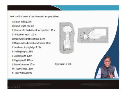
The dimension wise you can see, if you see the top view, it will be looking like that; the most important is that what is the total length on which it will be working, what is the total width it will be working and what is the total operating height it will be having and these dimensions it vary from make to make, you make a study of that.
