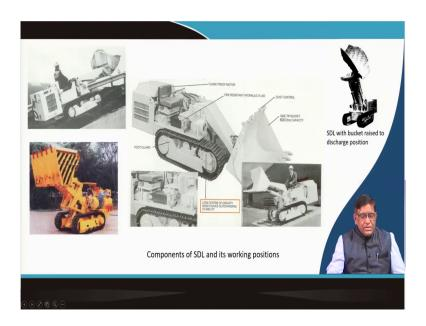
So, now coming to this exactly the components you have seen that, this it can work in a gradient; you can see that this is a side discharge loader working on a gradient. You can see here how the operators cabin is there and in that we can have that your ropes; that is your rollover protection system over here, then your this whole motor which is kept over here is a flame proof motor.
