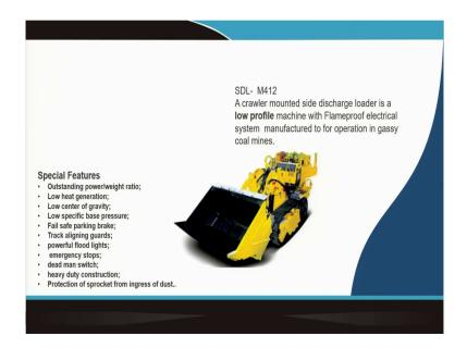
So, these are the machines which is used. And then the main features that is your special features is, it has got a very good power to weight ratio; that is a what is the total installed power in the machine and then what is the total weight of the machine, that is exactly one of the characteristics by which you judge a machine.
