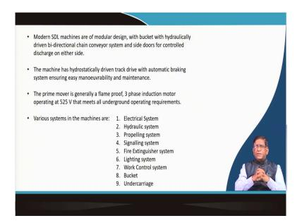
Now, there is a it is a, it this bucket of a side dishes loader, they can have inside the bucket there will be a bidirectional chain, by which the chain can move and then this material which will be collected in the bucket, can be taken out by the chain and then it can be discharged.
