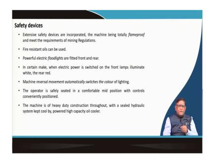
Now, this they as a safety devices, they have got a very powerful flood light; they have got excessive safety devices expensive extensive safety devices are incorporated in this machine so that no accidents take place and no fatality to human being or damage to the machines take place and for that, the fire resistance oil I have already told to you. Then there should be your, the type of light which will be used can be considered.
