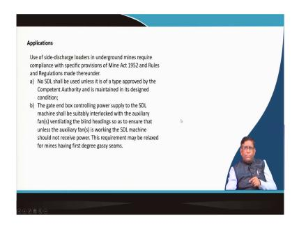
You please develop a write up how does an automatic disc brake work; because in the, we earlier discussed about the machine elements. Similarly, the applications of this is there in your underground coal mine will have to follow the rules; particularly in the mines act 1952, the rules and regulations are given for it should not be used unless and until it is an approved type by competent authority, you must mention that.
