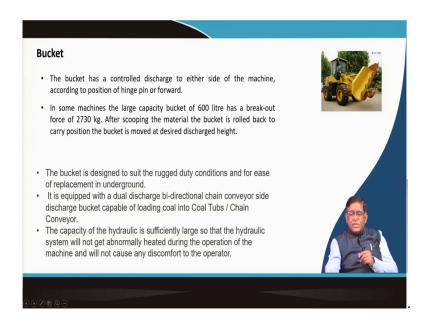
The bucket, you can see here is a special type of bucket, either without a chain you can see here, one side is open; you will have to while it is collecting, it is there as a reverse directions gradient will be there. So, that while loading, while bringing it over there, the material should not fall; at the time of falling, you can give by raising by one and the material will be discharged.
