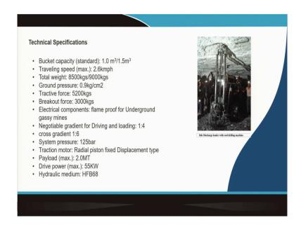
And you know that these machines can be sometime improvised that, machines can have attached it a roof bolting machines also; that is when the machine is working, collecting the material that it can give, it can drill upward holes are done by which you can just anchor, so that the protection of the roof can be given.
