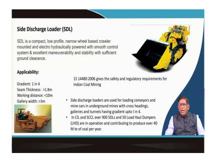
You can see here, that is the other machines other than this Rocker Shovel this; the next type of loader we are going to talk about is the side discharge loader. Now, when I talk about the side discharge loader; before that please clarify whether you have understood that, what is the loading machines purpose is.
