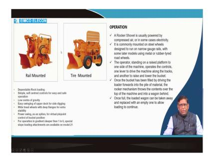
So, that we discussed about the gathering arm loader; here you are studying about these machines which is a EIMCO Elecon; they have manufactured these machines which has got a Rocker Shovel, which is this particular is a shovelling part and this will be working. You can see here is a one platform on which the operator can stand and then he will be operating these levers. So, by this operating this lever, this whole arm it will be going up above this once and then it will be discharging.
