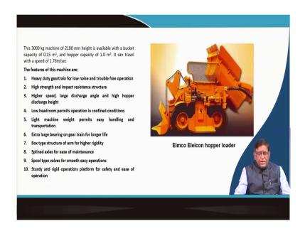
Now, you can see here that say, a EIMCO Elecon that the machines which this EIMCO produced in 1938; they have gone through different type of a developments over here. But today in this 21st century also, this machine is working and then this is the latest version of that machines which is shown over here.
