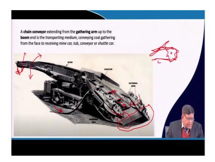
Now, let us see this machine first, what is this exactly. This is a machine for handling bulk material. We can say in underground mines this machine will have to work inside the mine that is your at the surface it is there it will go by shaft or then there will be there. So, this whole machine will have to be assembled down at a below that is in the underground.
