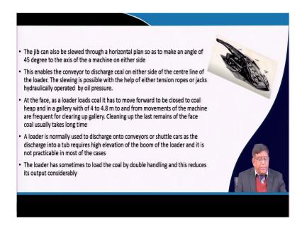
So, now you are familiar with this gathering arm loader; this is we can sometimes you can see the jib also. This front portions this also can jib also can give a slewing motions like that so that the collections can be better ok. So, this loading and unloading, and then the operations how you are giving, how much push you are giving this whole thing will be affecting the productivity of the system.
