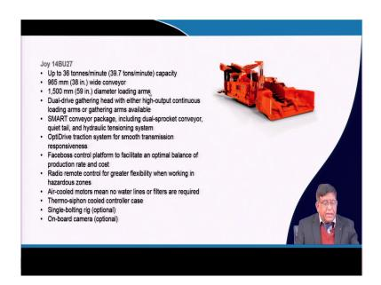
So, and then as in the previous figure I have shown you can start getting the some of the specifications. Whenever you are studying a machine you should try to understand the specifications exactly how to have an idea of the size of it. So, this is one particular model that is 14BU27 is a model manufactured by Joy company which is now taken and marketed by Komatsu.
