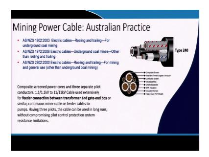
And, also you can see their constructions of those cables exactly in Australia also every country has got their standards. As per the Australian Standards they have got this Type 240, Type 241, Type 245 different types of cables for different type of use for different type of machinery.
