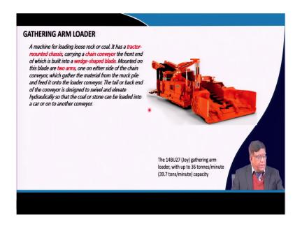
So, we will be discussing about these machineries. Now, what is that gathering arm loader which is it is a machine for losing that is it will be loading. Here you can see that this is the front part of the machines and this basically these machines comprises of this gathering head where there are some small arms the material is collected from these ones and then put into a chain conveyor. And, that chain takes the material, give it to a boom and a conveyor belt here and then the discharge boom.
