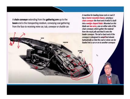
So, this is a as a this machine is for loading as you have said you can read this part that exactly this machine is for loading loose rock or coal. It has a tractor mounted chassis, that is, your crawler mounted chassis and it carries a chain conveyor at the front end.
