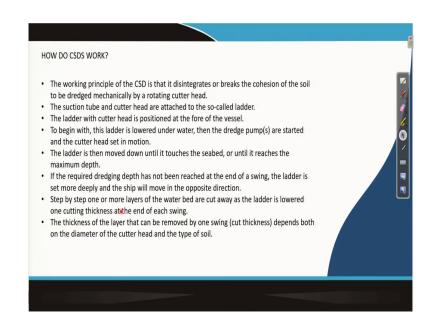
Now, this cutter suction this dredgers the cutter suction dredgers working principle is that it disintegrates or break the cohesion of the soil to be dredge mechanically by rotating cutter head.
