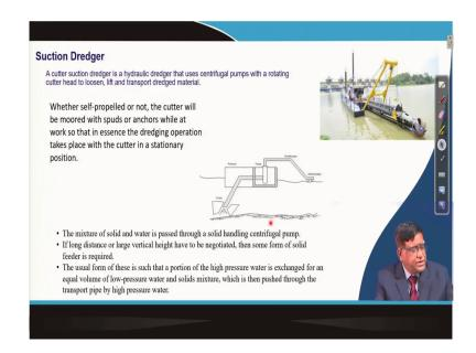
Now, this machine is a suction another thing is a suction dredger. The suction dredger, this you can see here there is a cutter and then this is a pipe through which exactly the pump will be here that pump will be pushing that material through this and then they will be processed over here and a material will be taken out of it.
