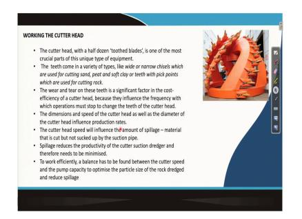
Now, they how the cutter head exactly work that is your it has got the toothed blades. You can see that blades that sometimes it is called toothed blades or peaks or cutting heads. Now, the this need to be replaced need to be maintained. Now, it is just like a chisel type of bit. So, that it can cutting sand, peat or soft clay, teeth. So, there if very hard rock comes and they get damaged then the wear and tear of this teeth is significant factor in the that cost efficiency of the cutter head.
