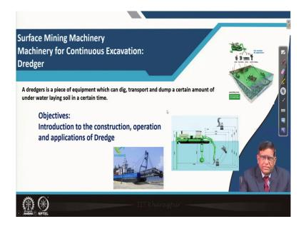
Now, today we will be discussing this dredger which is a piece of equipment which can dig, transport, dump a certain amount of underwater laying soil in a certain time; that means, this machine dredging machine it is main job is if there is a some rock surface or shell surface or anything is there which is below water it will be cutting from there.
