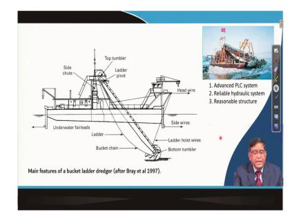
Now, you can see here what is this exactly a main features of a, that is your bucket ladder dredger. This is a ladder on which now this is a chain mounted just like a bucket chain excavator you have got this buckets will be cutting the bucket may be having the teeth and
