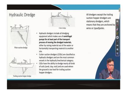
But in the dredging operations many of them they use the hydraulic dredge. These hydraulic dredge which can be a plain suction dredge from the below underwater, the material is exactly sucking through this and then through a pipeline as a slurry form and it is taking over there.
