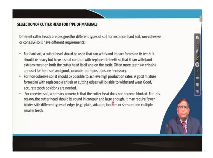
So, depending on the type of material you will have to select the cutter head. Now, different cutter heads are designed for different type of soil; for hard soil, non cohesive soil, cohesive soil they have got different requirements. For hard soil the cutter head should be used. So, that they it can withstand the impact forces on its teeth because hard rock it will be the impact will be more and then you will have to withstand that.
