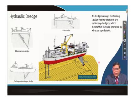
So, there is a different type of this dredges are available. This photographs give you a picture how a, it you can see a shape on which you are having a ladder at the bottom of it we are having the cutting head here. Now, this cutting head exactly you can see here this cutting head will be loosening the rock mass and it will be this ladder it can swing between this range so; that means, that this much part it will be cutting.
