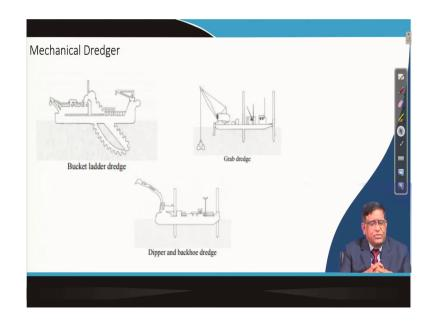
Now, if you think of this mechanical dredger it has got the bucket ladder dredges or it has got grab dredge and dipper and backhoe dredge that the photographs which I show in the first slide. It has a backhoe dredge or it can be a grab dredge. Sometimes it is also this type of this grab bucket excavators are used even its from some ship unloading they use this type of machines.
