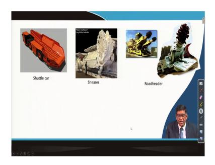
So, that is the different requirement and you can see here the wide range of machinery you can see this is the shuttle car used in coal mining, a shearer which is used in a coal long wall, coal mining, a road header which is main for performing the underground galleries or underground roadways are made by that.
