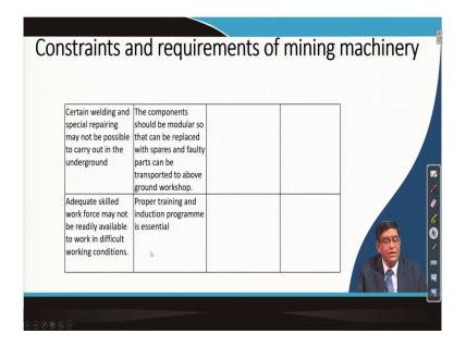
So, like that you can find out that is your what are the different type of requirements. For example, the adequate skill of the work force may not be readily available for doing that very specific case and very sophisticated machines to operate because many of the mines will be in a very interior area people are not well educated under that conditions you will have to find out that in which best way you can train the operator to do the machine.
