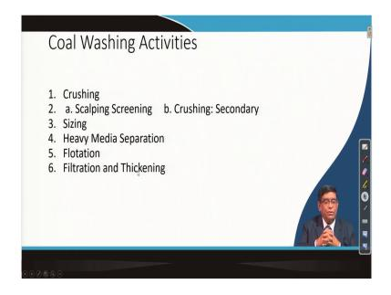
So, also we have got in case of coal mining there is a coal washery or coal washing activities are there and for that you have got a different type of crushers. There is a scalping machine, there is a sizing machines, there are heavy media separating machines, flotation selves and then filtrations and trucking.
