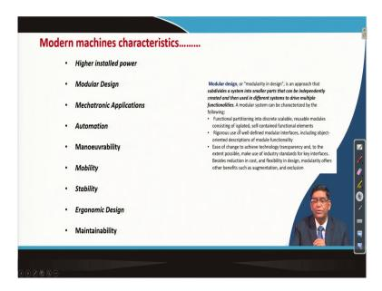
Then the modular design also I told you that it is then approach that subdivides a system into smaller parts that can be independently created and then used in different systems to drive multiple functionalities.
