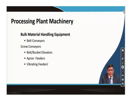
So, these main handling equipments are your different type of belt conveyors, there is a screw conveyors also there are apron feeder, vibrating feeders, feeder means by which you are feeding or loading the machines to the materials to another machine. Say for example, if your conveyor belt is running on the conveyor belt how you are exactly bringing the your other bulk material on to it that will be done by feeder.
