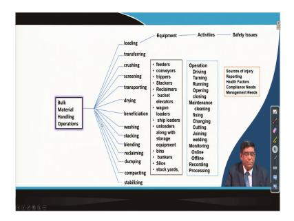
So, coming to this the bulk material handling operations in any miner mining industry is loading, transferring, crushing, screening, transporting, drying, beneficiating, washing, staking, blending, reclaiming, dumping, compacting, stabilizing so many actions. For doing these actions we have got different equipment, that equipments as a feeder, conveyor, stackers these equipments they do number of activities.
