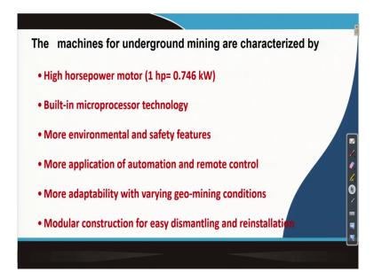
So, for an underground mining machines are characterized by very high horse power that is and then built-in microprocessor technology more environmental and safety features, more application of automation and remote control more adoptability with varying geo mining conditions, modular constructions. These are the things which are there.
