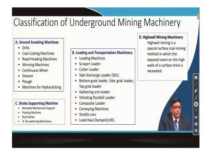
So, now whole these things you can see here as shown in a very specifically how different type of machines are there and then also we said that in the last class there is another class of machine called high wall mining machinery. In the high wall mining is a special surface coal mining method in which the exposed seam on the high wall of a surface mine is excavated.
