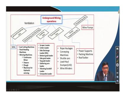
And, as I told you earlier also that these operations can be done by different machines like underground drills they have got you may be hearing one name called drilling jumbo that drilling jumbos are used for underground rock breaking. Now, for the developing phases for the in coal mining they used to use coal cutting machines now these coal cutting machines are now obsolete, but there are road heading machines which are working even more than 60 - 70
