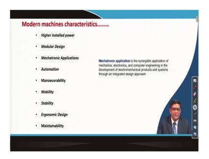
Similarly, in the mechatronic applications I have said it is a synergetic applications of mechanics, electronics and computer engineering in the development of our electromechanical products and systems through an integrated design approach.
