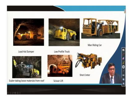
You can have this load hal dumper, that is used in underground metal mine also. And, this low profile truck that in underground space whatever is created within that the truck is there and this truck will have to be lifted to this the unload the material from here even sometimes in underground because of certain reason.
