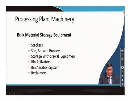
Similarly, bulk material storage equipment you have got this stackers, silos, bin bunkers, then from there how exactly you will be withdrawing those type of systems are also employed. And, then you have got the reclaimers; that means, once you have made a store, from that store how you are collecting the material.
