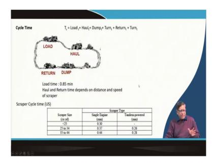
So, this is how things are done, and the total cycle time as I said that is different operations there all the time if you note it down, then you can find out what is the loading time and that is required to calculate the productivity of it.
