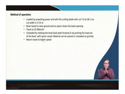
So, as a method of operation: loaded by propelling power propelling means the travelling power and with the cutting blade cut about 7.6 to 38.1 centimetre deep cut can be given with a 3 to 3.6 meter width that cut can be given. And, is a bowl is raised for the grounds and then apron closes and that it opens.
