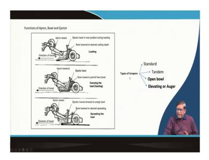
So, you can see that this how the functions are taken place over here. So, this apron which is exactly a gate for this for while this machine is moving in this direction, at that time your this blade is pushed you can see here, this is the level and here it has cut, so that level has gone down. So, this much when it is moving the material is going towards the back and it is getting filled.
