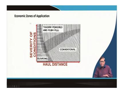
But, as a if your the severity of the site condition is very high, there your tandem and powered push pull those type of scraper will have to be used. If your haul distance is very long in there you cannot make in a very severe conditions and the severity is less and there your conventional scraper can be used.
