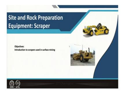
Now, this site preparation purposes though it is used, but it is basically a scraping machine, which is used for removal of the top soil. So, here we will be introducing this particular machine how it is used in the surface mines.
