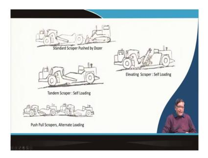
If you can see here in a standard scraper it can be pushed by a dozer. There is a dozer here and this dozer is pushing this material and then there is a tandem scraper means you have got one tractor engine here, one engine here at the back, so that the required power to cut, and load, and carry that is given by two.
