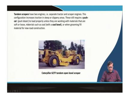
Now, you can see here a photograph of a Caterpillars, Caterpillar tandem you can see here is also the one engine, one engine here in the centrally that bowl is there. So, this type of machine can take this your top shell can be removed and put it over there.
