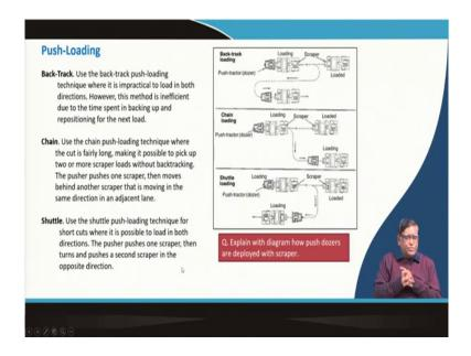
So, now when you are doing it is a push loading you can give that as a back track loading. Now, you can see in this diagram a dozer is here to push the scraper and then it gets loaded and then it just coming and that getting spreading.
