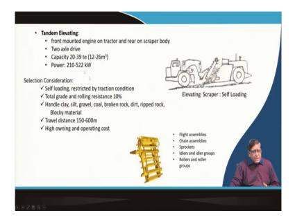
So, this in the elevating here also your a front mounted engine is there and here the capacity can go 12 to 26 meter cube is a small capacity, but it is a self loading. So, that is it is getting a properly loaded. So, bowl get properly filled and that is why the machines the productivity can be little more.
