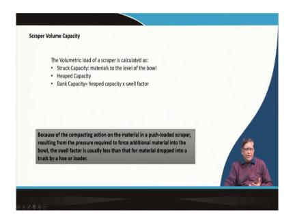
And, the volumetric load on the scraper it is calculated as a struck capacity. Struck capacity means, when you take a water in a glass, then it is just up to here that is just struck capacity, but on a glass if you put rice there will be a heap capacity. Some material can depending on the angle of repose it can be kept over there.
