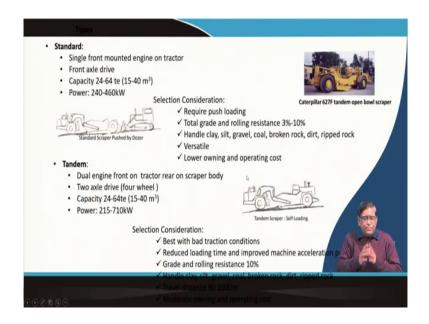
Now, if we see there in a standard scraper, the single front mounted engine on the tractor is there and drive is a front axle drive and its capacity goes to 15 to 40 meter cube is the bowl capacity and for that the engine need to be of 240 to 460 kilowatt that is the range available in the market.
