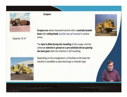
So, now what is a scraper? So, this scrapers are basically a wheel mounted machinery that is a it is a off highway wheels large diameter wheels, which are that is a wheel mounted machinery working in the mining field and it has got a centrally located bowl.
