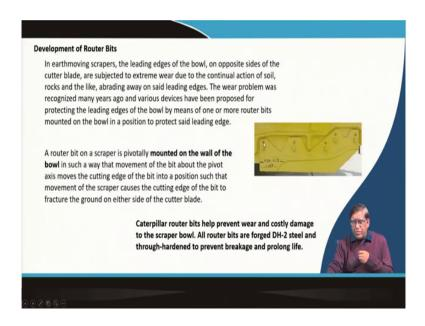
Now, there is another things that router bit because what happens here the blade this edges will get worn out. So, that is why to protect that there is a router bit over there that you can see at the in front of the cutting blade an another bit is being from the side walls fixed.
