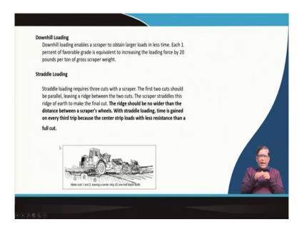
So, it is it can also while you can spread it in downhill, it can cut also downhill depending on the site situations you can find you can determine that is exactly, but a 1 percent gradient is considered as a favourable gradient. If you put it over there it is exactly get a better cutting and better hauling things.
