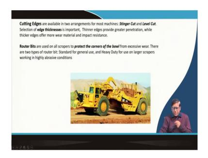
So, this is the cutting edge which is there you can see how the material get loaded over here and there is a guard by which the material should not get spilled.
