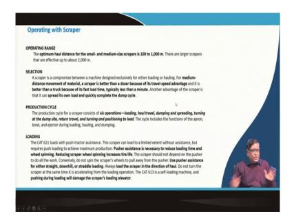
So, while you are to these machines now you have understood that, what is a scraper-scraper is having a bowl at the central at the bowl. There is a teeth for cutting the or blade for cutting the rock, there is an apron for holding the material and there is a hydraulic arrangements for raising and lowering of the apron, raising and lowering of the teeth and also for the articulations and sometimes you are having this elevator.
