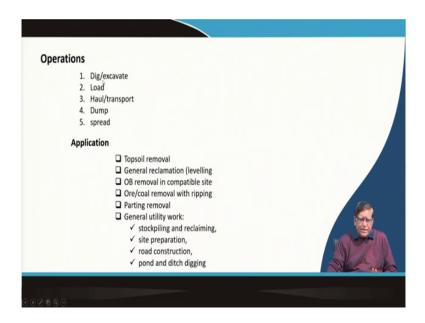
So, they as I have said already the operations are digging, loading, hauling, dumping and spreading. Its main application area is topsoil removal, general reclamation, over burden removal in compatible sites, then it can be also parting removal can be done.
