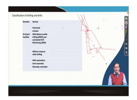
Now, if you do a drilling very straight over here what happens; when you put the explosives and you want to do the blasting here your the burden becomes more. So, that is why sometimes the drill hole need to be made at an angle drilling this is called your angle drilling.
