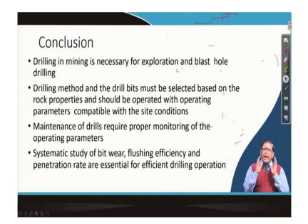
So, in a mines when you want to do a drilling operations or you need to understand that different parameters effect right from the; how the machine is designed, what are their parameters and then how it is affecting. When you can correlate them; then you can go for a really advanced or that automated mining automated drilling operations your automated decision making.
