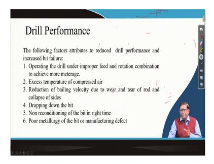
So, normally for each particular diameter of the drill hole you will have to have a specific axial thrust and a specific RPM under that combinations. And then how at what speed you are taking out the material that will be giving you the optimum penetration rate. If you are making a very fast drilling, but you are unable to take out the debris then your rod will get jammed. So, those type of drilling problems take place.
