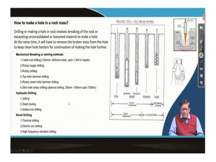
So, coming here; you can see that you can how we make a hole in a drilling or in a rock mass. So, there we will have to be you will have to dig a hole. Digging a hole means you are removing some material from here. So, the basic principle of drilling is what? We will have to disintegrate this rock mass over there.
