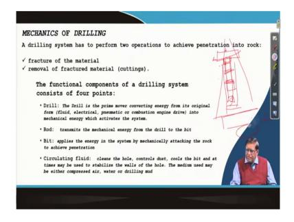
Or your when you are having a rotary a bit is there you are giving an axial thrust on it and then with this thrust you can just exactly in while doing this job you can see here you are giving a thrust over here and then you are rotating this. At this what is happening that under this axial thrust you are allowing a force to go get into this rock mass and with the rotations it is breaking the rock.
