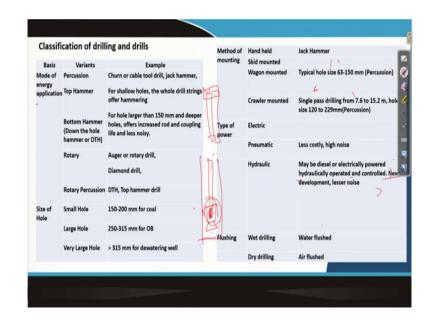
Now, if we see that there is a various way how you can classify the drilling. You can classify on the board on the mode of energy application which can be a percussion. That percussion can be given; that means, your the rod is here and that rod can be given from the top it can bring or the rod below the bit is there and only the bit part is moving.
