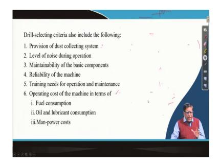
So, just a drill how we will be selecting for a particular area that whether you are doing an iron ore mining or bauxite mining or coal mining. What type of drill is required that selection is a lot of this data whatever related to the machine parameters and related to the rock.
