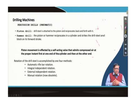
So, what is this when we say about the pneumatic drills or the percussion drill. The percussion action is given by compressed air. So, here that we say the drill steel; drill steel is the rod on which you are having at the tip the bit the bit could be a cross bit or chisel bit by which is an integral part of the drill steel and it is exactly the action is given by a piston actions.
