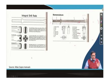
So, now as we have said that integral drill rod in percussive drilling that we are having a hexagonal drill rod like this at the end of it this is your tungsten carbide button is inserted this is called your chisel bit. And that this can be given as a two then it is called a cross bit.
