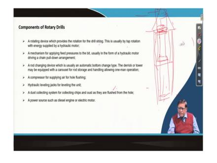
So, this rotary drills can that is your the component wise it has got a rotary device by which the rotations will be given there will be a mechanism for applying these feed pressures. There will be that how the rod because when you start doing the drilling after doing one drilling then your rod will have to be taken up.
