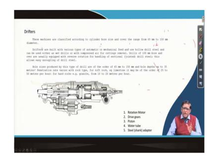
So, this is how that the drifters also another type of your percussive drill which is also used in underground coal mining sometimes in a say when there is a the rock is to be drilled through there they use this drifter it is also principle is same by controlling the valves you are giving a percussion actions.
