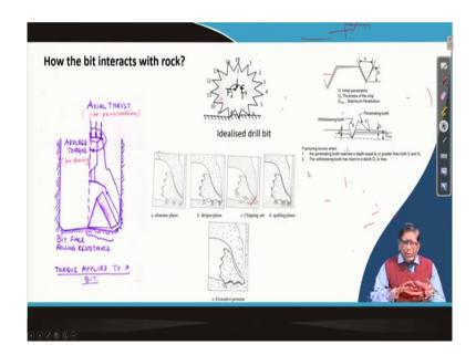
So, the rotary drilling when it works exactly the tricon roller bit. We have already discussed in the how it interact exactly on the axial thrust and then a torque is applied and this break is the rock is broken. It is just simulated as a cutting a idealized bit is nothing but a treated wheel when it is going it is under the under the axial thrust.
