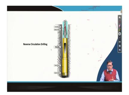
So, this is then the other thing is rotary drilling can be a reverse circulation drilling where that drilled rod your fluid is not coming through the drill rod over here. Fluid is going through the annulus and the debris is going through this rod and that is connected collected.
