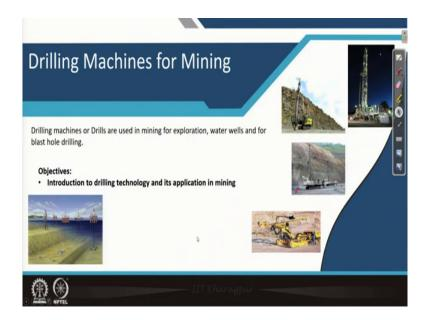
Now, this say drilling machines they are used widely a quite a large varieties of drilling machines are there. As you can see these photographs here this is a drilling rig in the oil industry and also in the mining industry you can see these are the blast hole drilling of different types. Here that there are mainly hydraulically operated a percussive drills or the drilling is also in the offshore where they do for the drilling for oil wells below the seafloor.
