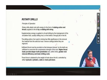
So, similarly in your rotary drill you are you can see here a drilling rig in a oil well drilling such type of rotary drilling will be there. Where there will be a crown on which this wire rope will be holding this whole thing is called drill string number of rods they are connected with this that is called sub or they are coupled together.
