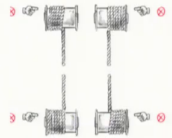
left hand drum - right hand lay rope If you move your finger counter-clockwise, drum (reeving system) is left hand, and needs right hand lay rope.
