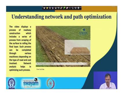
So, let us observe one video at this moment so that which is taken from the YouTube so that we can understand, this is a road construction process, you can see first the vegetation is removed, then the first soil cover is rolled, then the metallic cover is given on that, then the coarse aggregates are placed on that. Then finally, the rolling of the coarse agreements are given that is the GSB layer granular sub base layers of after
