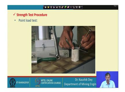
The test part with marking the center point on the samples by using a pencil and ruler, find a midpoint of the top sample based on this causation line. And with the same thing to the bottom one, this is important in order to get a good result and through mode or failure.
