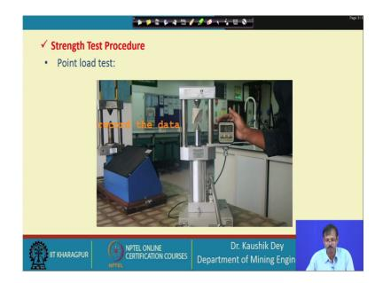
Then place this rock sample in between the sharp edge and you can see here bottom and top edge. Then give a little pressure so that the sample is properly located and cannot move anywhere.
