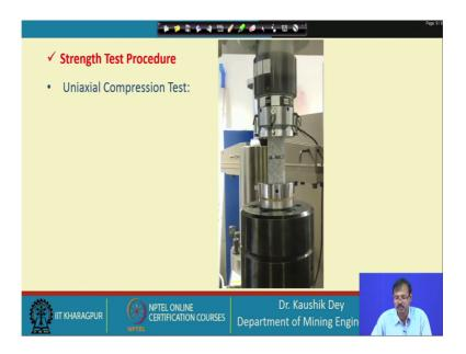
In this test you can say this is the one video of the test; in this test you can see the loading is being carried out for a compressive test sample. So, this sample is placed there is no eccentricity the plates are parallel to each other, while it is under loading. And gradually with a fixed loading rate the load is being increased on the sample.
