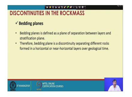
But the important is that the joint and bedding planes, these are commonly observed and that need to be taken care bedding plane is defined as the plane of separation, between two layers of different material and also the static considered as the stratification plane.
