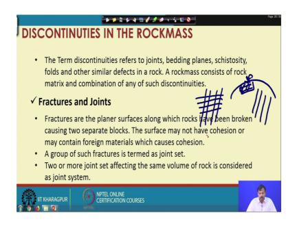
Now, let us understand about the properties of the rockmass, the rockmass property which is basically very very important for our drilling and blasting, purpose those are the property is called discontinuity properties of the of the rockmass. This term discontinuity refers to the joints bedding, planes, schistosity, joints bedding, planes, schistosity folds faults. So, these are the basically discontinuities, which are considered the dictating the properties of the rockmass.
