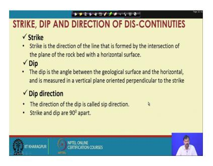
So, that is why the direction of dip directions are also very very important for our as the rockmass property in rock excavation part, specially in this course where we are dealing with the drilling and blasting. Dip direction is the direction of the dip is called dip direction a strike and dip are 90 degree apart.
