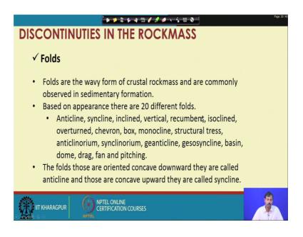
The major property which needs to be considered is the joint set not the fault. Similarly, faults are also there which is basically; wavy form of crustal rockmass and are commonly observed in sedimentary formation and, based on their appearance, it can be divided into anticline syncline like different types of classification.
