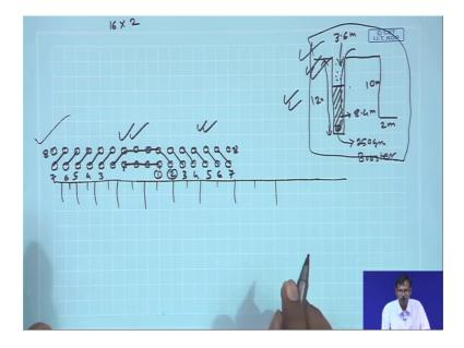
So, there are 16 into 2 holes so, let us consider this is the free face and these are the holes 1, 2, 3, 4, 5, 6, 7, 8, 9, 10, 11, 12, 13, 14, 15, 16 holes then 1, 2, 3, 4, 5, 6, 7, 8, 9, 10, 11, 12, 13, 14, 15, 16 holes of 2 rows and you have to blast it in extended V cut pattern.
