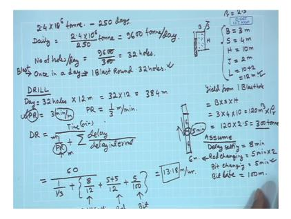
Our yearly production target is 2.4 into 10 to the power 6 ton, which has to be achieved in 250 working days. So, our daily production target daily production target is 2.4 into 10 to the power 6 divided by 250 ton. So, this is if we calculate it, it is coming 4000 here at this place into 2.4; that means, 9.6 into 1000. So, 9600 ton per day is the production target.
