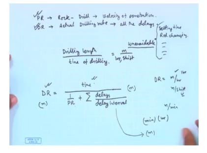
So, basically penetration rate which is nothing penetration rate which is nothing, but the interaction rock drill interaction depends on that the penetration rate is nothing, but the velocity of penetration whereas, drill rate is basically the actual drilling rate which is achieved considering all the delays which are unavoidable. So, this setting time, setting
