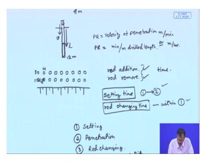
So let us see, in this case if you are considering that if this is the hole to be drilled by the drill machine the speed at which, the drill bit is moving inside the rock mass is called penetration rate.
