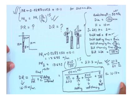
So, this property this formula which is given the penetration rate the penetration rate is given as the formula, 0.0283 uniaxial multiplied by uniaxial compressive strength plus
