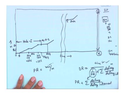
So, this is the basic idea about determining the penetration rate and the drilling rate; however, let us understand this in a better way if we draw the time diagram for this. So consider, consider this is the meter of drilling and this is the time. So, let us consider at zeroth time, we start our machine and we need as we have discussed, we need 8 minute, we need 8 minute to set the machine on it is own position.
