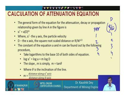
So, basically this dependency we have converted by taking this log in both the side in a linear form, so that if we are having a data PPV, then say R by root W let us consider this is the D. So, if we are having this value, then after that we go for taking the log value of this one. So, let me erase this one.
