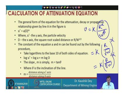
What approximation carried out in this, see as this is in last class we have seen, this is a sinusoidal wave, we are measuring the velocity. And as per our dependency, we have found that velocity is proportional to K may be R to the power alpha or W to the power beta that may be the some understanding, which is carried out. In the previous slide, we have seen different dependency of this alpha beta is proposed.
