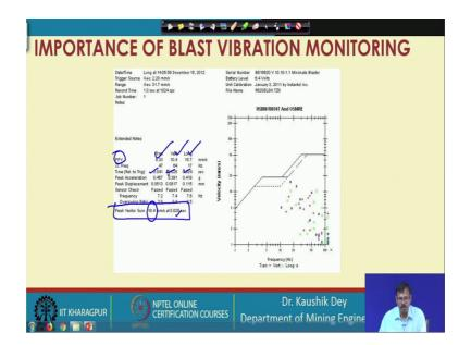
However, the structural damage etcetera are dependent on the velocity, not on the acceleration. So, in general, you can have a peak particle velocity value from the report of the seismograph in each channel it is given, its time of occurrence is also given in each channel. You can see the peaks are occurring at different times, it is 0.24 millisecond for longitudinal, vertically it is 25 millisecond, and 41 millisecond for the transverse.
