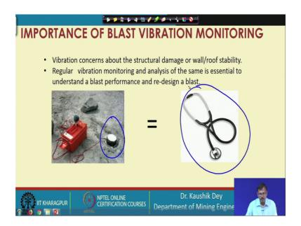
However, blast vibration monitoring is very very important, because personally I believe the blast vibration monitoring which is carried out by a seismograph is more or less similar to a stethoscope for the blasting engineers. So, a seismograph observing the result of the seismograph that is the blast vibration in a time scale or the oscillation of that particular point in a time scale, a blasting engineer may draw a number of conclusion, and the blast may be re-designed based on that.
