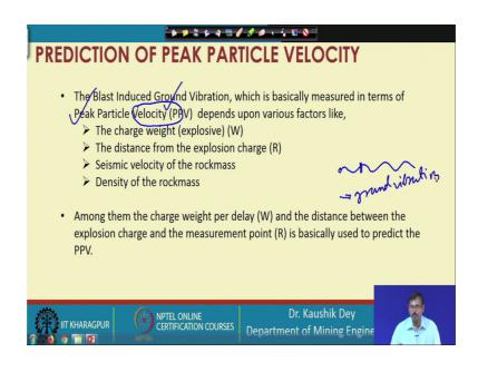
In mining purpose, while we are basically define our ground vibration, we express the vibration in terms of velocity in terms of velocity. So, basically we are interested in the measuring of the velocity of the oscillation of the particle with respect to the time. So, this is the major measuring technique and we found we have found that this velocity, the
