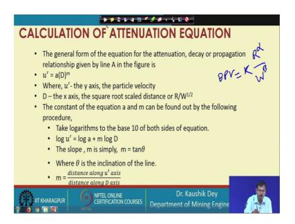
And we can now go for PPV is equal to K into R to the power alpha W to the power beta, which is basically the generalized equation for the blast vibration prediction.
