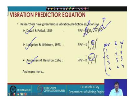
And different researchers, researchers have proposed different predictor equations for blast induced ground vibration. And you can see the Duvall, Petkof as are good for square root scaling distance, this square root scaling distance for the peak practical velocity analysis. And they have are good two constant, these two are site specific constant, this is propagational constant, and this is a site specific constant or you can say rock constant.
