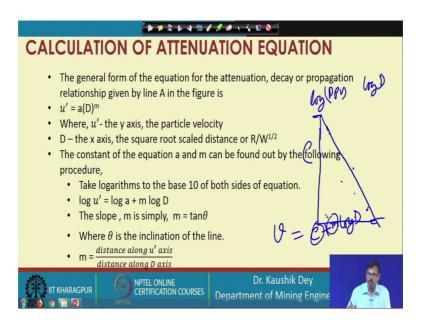
Then we have to compute the log PPV and log D value, then whatever value will be observed. After getting this value if we plot a line in between this, we will get a C value, we will get a C value here, and we will get the slope of this one and we can plot considering this, we can get the equation v is equal to c plus into m. So, this c and m value can be computed very easily.
