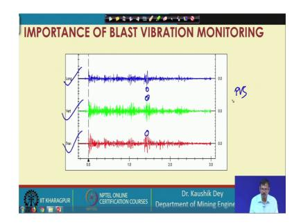
This is more or less an output, which is observed from a vibration monitoring. And you can see in last class as we have discussed, the monitoring is carried out in three channel; longitudinal channel, vertical, and transverse channel. In longitudinal channel, the sensors are facing the blasting site. Transverse is the perpendicular to that and vertical is the vertically perpendicular to that direction.
