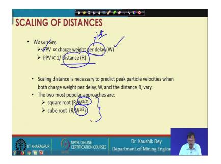
So, with this consideration, researchers have found that peak particle velocity that means, peak magnitude of the ground vibration in term measured in terms of velocity is directly proportional to the charge weight per delay means at that particular instant at that particular instant, and it is inversely proportional to the distance. So, this is very very important point that it has been found, it is proportional to the charge weight, it is inversely proportional to the distance.
