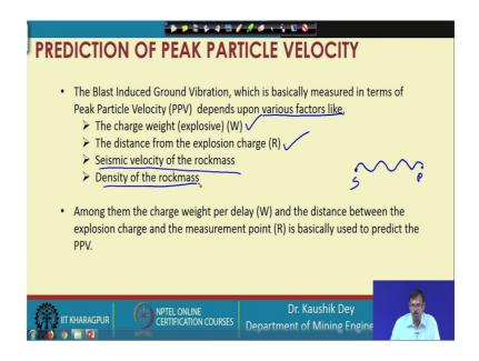
And we are interested the peak value of that velocity considering the stability of the ground or the compactness of the ground, so that we can find out how much magnitude of vibrating ground vibration is being generated because of blasting up to a sensitive structure or up to a point of interest. And it has been found a various factors are affecting that one.
