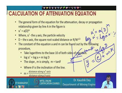
So, if you carry out this the same writing D to the power m and take the log in the both side, you will find log u dot is equal to log a plus m into log let me rewrite it plus m into
