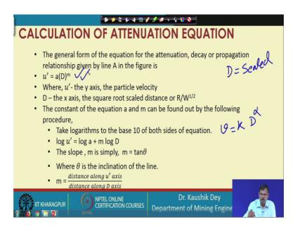
And this R by K R by root over W or whether it is R by cube root of W, it is considered as a D, which is called scaled distance; and this scale distance may be square root cube root or may be n number of variations are there as we have observed. So, it has been found the velocity is proportional to D to the power alpha, which is expressed as this in this case.
