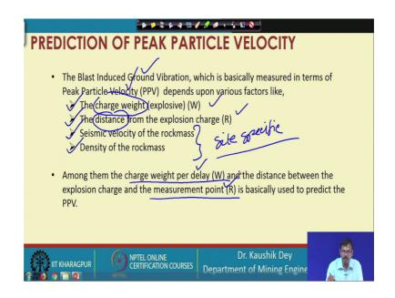
Charge weight or explosive charge at that particular instance, then the distance from the charge explosive explosion charge to point of interest, the medium characteristics, and the again the medium characteristics, so these are very very important. And it has been found by the researchers that if we are considering the charge weight and the distance as two variable, then the rest two part may be taken care of well by some site specific constant.
