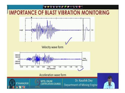
This is this slide is basically showing you the difference between this is the velocity wave form. For the same blast, if you go for the acceleration wave form, you will find out this one. I have tried to place it in a same scale, but I think it is scattered a little bit. So, this point is at this position this point is at this position, so it is little bit scattered, but if you can see the it is more or less this one is more or less similar, so this part is belongs to this part.
