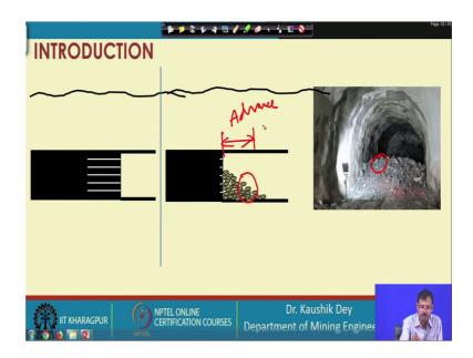
So, our objective of fragmentation objective of fragmentation and objective of hole utilization factor or advance is very important.
