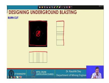
Empty holes, then the explosive loaded holes and this empty hole is basically act as the free face for this loaded holes. So, if we are asking this one first, if we are blasting this
