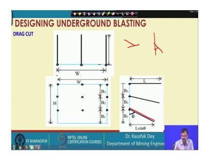
And, if you just tilt it 90 degree. So, that the wedge angle is becoming creating an wedge with the horizontal, creating an wedge with the horizontal then it can be called as drag
