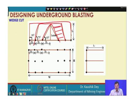
So, for this hole this will act as the burden and a free face like this will be observed after this blasting. And finally, a free face like this one will be observed. Basically in our design consideration we have already discussed, that fan cut and drag cut is basically up wedge cut.
