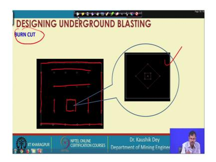
So, now let us consider about the different designing theorem. We are having one burn cut designing theorem, in which the holes are drilled parallelly and all the holes are horizontal there is no angled holes. And, we have already discussed this case in case of our drilling consideration. So, I while we have carried out our drilling patterns for the underground miles and that term we have already discussed how the burn cuts are there?
