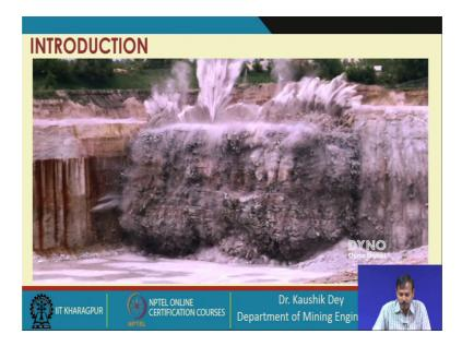
Here, also you can see little bit in few holes, stemmings are ejected; but mostly, we can see how the explosive a fragmentation is carried out. Then the fragmented rock is being thrown using the explosive gas pressure.
