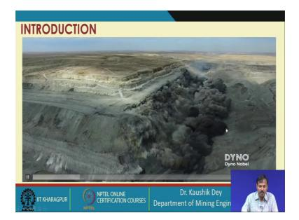
So, this is absolutely considered to be a very good blast because there is no stemming ejection. Stemming is completely successfully carried out; only the throw of the material is carried out in the front direction; only the throw of the material is carried out in the front direction.
