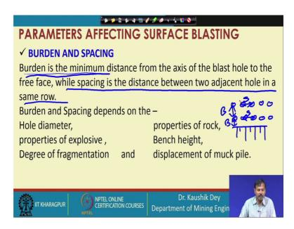
So, we are now discussing the Affect of Burden and Spacing on the surface blasting. So, burden is the minimum distance from the axis of the blast hole to the free face as shown in the previous picture. While, spacing is the distance between two adjacent holes in the same row.
