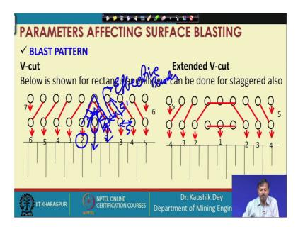
V-cut blast pattern is also another type of blast pattern, where you can see this is the Delay number 1; first hole is being blasted here as this hole is blasted.
