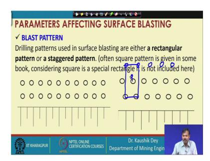
So, basically if you are considering this much of area, you are you will find there is a central location of hole which is basically giving the charge concentration centrally. So, the charge distribution may be better in case of staggered drilling pattern than the rectangular drilling pattern.
