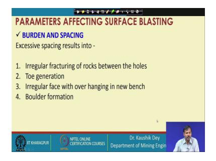
So, excessive spacing result into Irregular fracturing, Toe generation, Irregular face with over hanging in new bench and Boulder formation. So, these are the results of excessive spacing if we are poorly design it.
