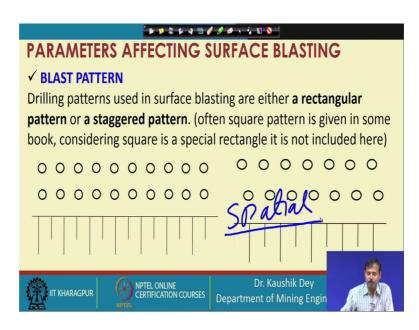
So, in other words, you can say the spatial distribution the spatial distribution, the spatial distribution the of explosive is better in case of staggered drilling pattern than the rectangular drilling pattern.
