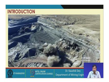
And you can see the delay of those different holes on which those are blasted, those are also easily observed. Because this is this video is taken in a high speed camera and it is now showing you at a lower speed. So, that is why the movement of the shocks etcetera can easily be visible through our naked eye.
