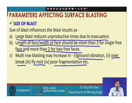
Next is size of the blast. Size of the blast basically dictates with the number of rows, number of holes per row and large blast reduces the unproductive time due to the evacuation which has to be carried out during the blasting. The length of face by width of the face should be more than 3 for a single free face and should be more than 2 for two free faces. Multi row blasting may increase in the ground vibration because of the improper burden movement, over break, fly rock, poor fragmentations.
