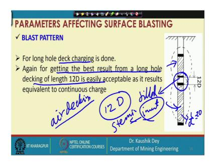
So, in charging pattern we can have our modification on that. For a very long bench height instead of having l by D ratio more than twenty we may reduce some explosive consumption by providing a gap in between.
