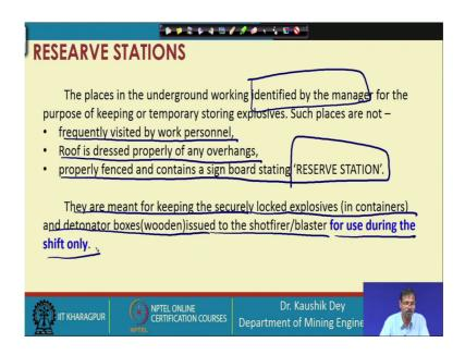
This must be identified by the manager, and mark it as the reserve station. This reserve station must be frequently visited by the work personnel so that pilfering of the explosive cannot be done roof must be dressed properly there should not be any overhangs so that that will fall on the explosive and give the shock for the premature blasting of the explosive.
