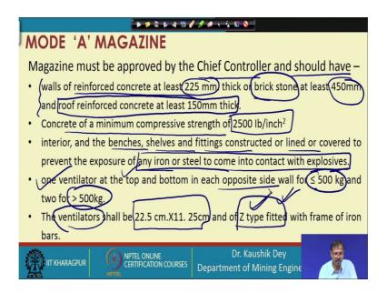
So, let us discuss about the first magazine, that is the first type of magazine that is the mode A magazine. So, mode A magazine is the magazine and this is of very large quantity of quantity of explosive can be stored in this magazine. And this type of magazine must be approved, must be approved by the chief controller of explosive. And this type of magazine should have walls if it is of reinforced concrete, then the concrete
