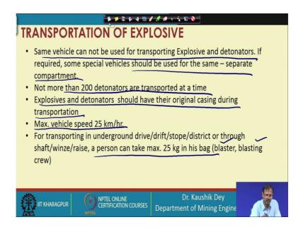
Same vehicle cannot be used for transporting the explosive and detonators. If required special vehicles may be manufactured where the separate compartments are there for the explosive and detonators not more than 200 detonators are transported at a time. Explosive and detonator should have their original casing during the transportation. So, it is not that, it has to be taken out from the original casing and placed in some other casing.
