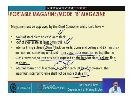
Now, let us look into the portable magazine or mode B magazine. So, mode B magazine must be approved by the chief controller of explosives, and should have the wall of steel plate. So, these are portable magazine. So, this can be moved from one place to another place. So, that is why this will be made of steel plate of at least 5 mm thick.
