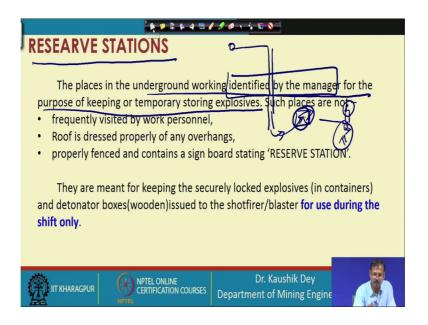
Reserve station is also another type of storage place very, very temporary this is very, very temporary storage place of explosive in the underground. The places in the underground working identified by the manager for the purpose of keeping temporary storing of explosive; that means, if there is no underground magazine, the explosive is taken from the surface, then through cage the explosives are transferred to the underground.
