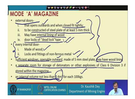
Second next requirements are the doors. There must be a door to enter into the magazine. The door must open outward. We have also seen in the video that door must open into the outward. And it should fit tightly; that means, there should not be any gap between the doors and it is frame so that anyone can be sent through that gap.
