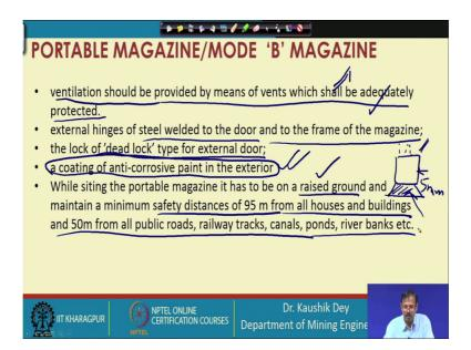
Again we have to provide the ventilation. We have to provide the ventilation by means of vents. And this vents should be of adequately protected. So, these type of vents are in general provided so that no one can send anything inside through those vents. And that is why inside is it will be a protected. External hinges of steel welded to the door and to the frame of the magazine.
