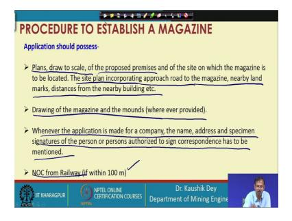
Now, the application should have all this applications for granting the license of explosive should have a plan of the proposed premises. That means, on the land on which the magazine has to be built up that must be plan and a sections of that area must be given or must be a enclosed with the application. The site plan incorporating approach road to the magazine nearby landmarks distances from the nearby buildings, roads, etcetera must be there in the plan.
