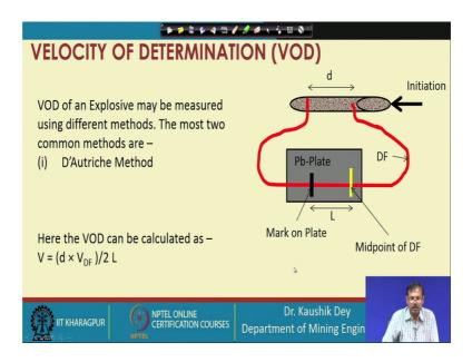
How we can measure the velocity of I think there is some problem in the slide please correct it, this is the velocity of detonation. So, this is the velocity of detonation. So, velocity of detonation of an explosive may be measured using different method. So, in this class we will discuss more most common two method; one is the D'Autriche Method, which can be applicable in the laboratory condition.
