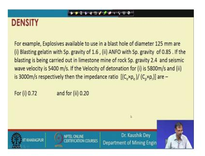
The third point which we are discussing that is the transfer of energy from the explosive to the rock, you know in a blast hole if we are considering this is a blast hole and we are placing our explosive column on this. The moment we provides some initiation in this explosive column, the first the shock is extracted from the explosive.
