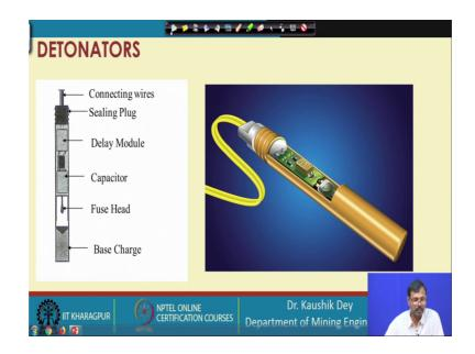
Let us see the construction nitty-gritty of this; you can see the delay detonator the delay detonator of electronic type basically taking the current from the lead wire. Then in that current there is a delay module provided ok; that means, it is the electronic delay programming said that the delay is provided in the movement of the electrical pulse.
