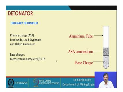
So, let us see the constructional utility of the Detonator this is the ordinary Detonator and in ordinary Detonator you can see this is a plastic tube, in this plastic tube the first primary explosive charge is kept.
