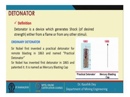
So, first let us start with the first let us start with the Detonator. So, what is Detonator? Detonator is basically a device which generates shock either from a flame or from any other stimuli; that means, we generate a shock or we convert the flame to the shock in this device. So, basically Detonator is the device where either we receive a shock or we receive a flame and that is converted to the desired amount of shock which can be considered as the significant shock to explore the explosive.
