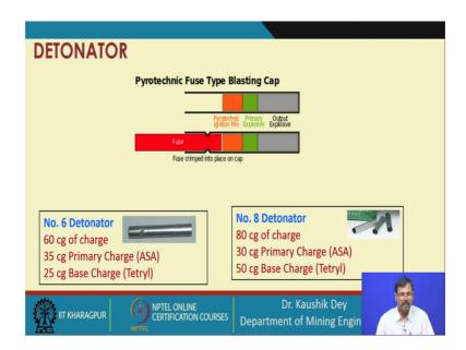
So, basically what we do in this ordinary Detonator, we keep the Detonator we provide some something which takes the flame from the outside and comes be in touch with the first primary charge and that primary charge is ASA.
