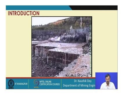
Then it will be shown in a slow motion. So, that how the Detonation has been carried out you can understand see the time gap which will show you the Detonation has been started from the left side, and it is gradually shifted towards the right side and the holes are accordingly blasted. You can see the similar video for the next blasting also.
