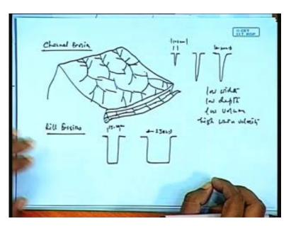
Since, they are of low volume, they are of low volume, they allow water to flow, they allow water to flow in high velocity, they allow water to flow, the rain water to flow in high velocity,
