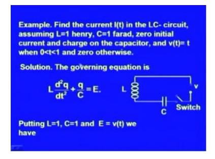
So, let us begin with a problem on electrical circuit, let us find the current I t in the L C circuit, here we are considering only I t, I c, L C circuit, r is not there that is resistance is not there. We are assuming L to be of 1 Henry, C to be of 1 farad and with initial current 0 and initial charge on the capacitor also 0. And we are given that v t is equal to t, when
