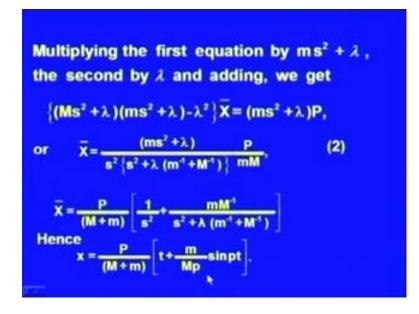
Now, we multiplication by m s square plus lambda the second by lambda and then add this by doing this, we will be eliminating 1 variable that is Y bar and we shall have this equation in X bar. So, M s square plus lambda into m s square plus lambda minus lambda square into x bar equal to m s square plus lambda into P.
