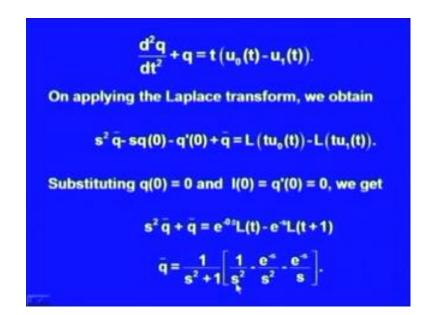
So if we do that we will have the differential equation like this d square q by d t square plus q equal to t times u naught t minus u 1 t. Now, let us apply Laplace transform to this equation L of d square q by d t square, we know will be given by s square q bar minus sq 0 minus q dash 0, then L of q is q bar and then we have Laplace transform of t into u naught minus Laplace transform of t into u 1 t.
