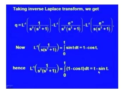
Now, let us take the inverse Laplace transform of this equation, left hand side will give us q and the right hand side using linearity, we will have q equal to L inverse of 1 over s square into s square plus 1 minus inverse transform of e to the power minus s over s square into s square plus 1 minus inverse transform of e to the power minus s over s into s square plus 1.
