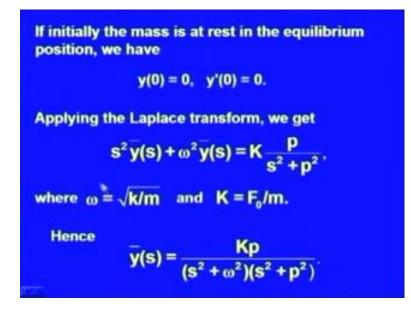
Now, we are assuming that initially the mass is at rest in the equilibrium position, so we will have y 0 equal to 0 and y dash 0 equal to 0. And, when we take the inverse lap when we take the Laplace transform of the governing equation of motion of the mass m we have s square y bar s plus omega square into y bar s equal to K into p over s square plus p square, where we have assume that omega is equal to square root K by m and capital K denotes F naught over small m.
