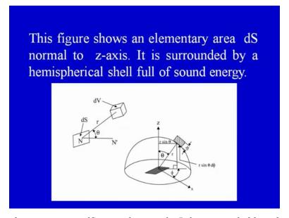
This figure shows elementary area dS normal to z axis. It is surrounded by a hemispherical shell full of sound energy, diffuse sound energy.
