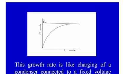
This figure shows the growth. It is like charging of a condenser connected to a fixed voltage source through some resistance. Let us now consider a decay of sound energy,
