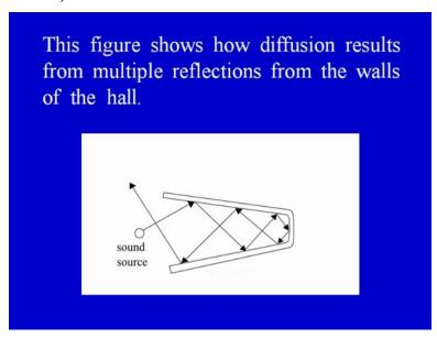
The figure shows how diffusion results from multiple reflections from the walls of the hall.
