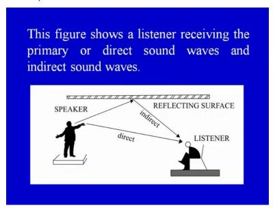
This figure shows the listener receiving the primary or the direct sound; sound waves and indirect sound waves.
