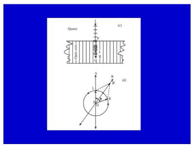
Consider some point PQ in the figure, in a right handed crystal along the path of a plane polarized incident beam.
