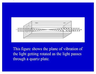
This figure shows the plane of vibration of the light getting rotated as the light passes through a quartz of a quartz plate. Remember, the propagation is along the optic axis.
