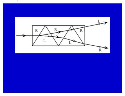
Alternate arrangement of right-left, right-left like this and the plane polarized incident beam.
