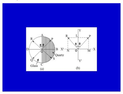
This device consists of a semicircular half wave plate ABC of quartz cut parallel to the optic axis as shown.
