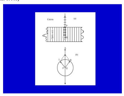
The upper part of the figure shows the propagation of the circularly polarized to beam.
