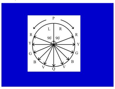
L for the left handed quartz and R for the right handed quartz joined along the diameter PQ.
