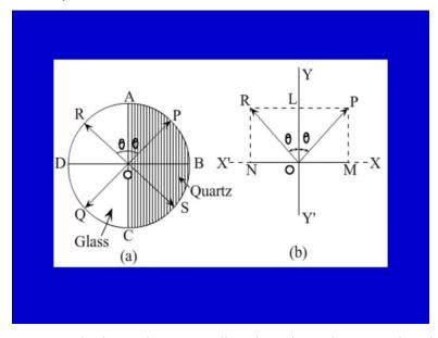
The two components travel along the same direction through separation but with different velocities. The ordinary component moves with greater velocity than the extraordinary component.
