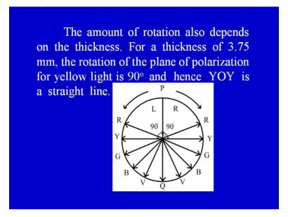
The sense of rotation is opposite in the two halves. The amount of rotation also depends on the thickness. For a thickness of 3.75 millimeters, the rotation of the plane of polarization for yellow light is about 90 degrees. And hence YOY is a straight line.
