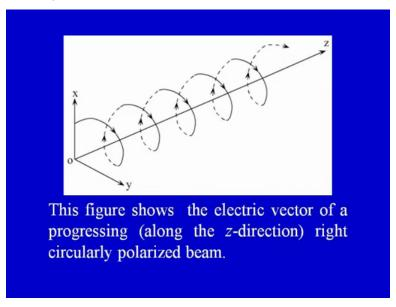
This figure shows the electric vector of a progressing right circularly polarized beam.
