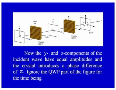
So, the ordinary and extraordinary again have equal amplitudes. The crystal introduces the phase difference of PI. Let us not consider the quarter wave plate part at the moment. Just for the emergent light beam in this case we have,
