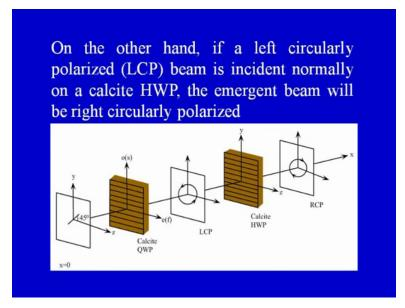
Now, on the other hand, if your left circularly polarized beam is incident normally on a half wave plate, the emergent beam will be right circularly polarized; initial plane polarized light passes through a quarter wave plate becomes a left circularly polarized light passes through a half wave plate becomes right circularly polarized light.
