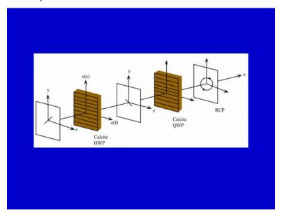
The incident light with a plane polarized with angle of 45 degrees passes through a half wave plate. The phase difference becomes 135 degrees passes through quarter wave plate which introduces another phase difference of Pi by 2. And the result is the light wave right circularly polarized.
