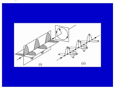
The figure shows the progressive phase difference between the ordinary and the extraordinary beams.
