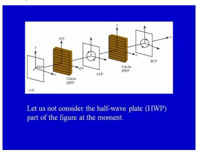
The passage through the quarter wave plate makes the initially plane polarized light. With equal amplitudes, the quarter wave plate introduces a phase difference of Pi by 2, of quarter vibration the result is we get a left circularly polarized light.
