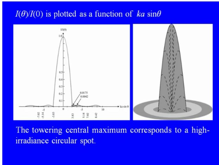
Here we have a plot; you see this on the right side this towering central maximum corresponds to the higher radiance circular spot, carrying an intense total energy content of 84%. Then it shows a ring, second ring. On the left we have a graphical picture, showing the intensity of the central maxima and related to that, we get a minimum at 3.83 then we get another minimum at 7.02 really 7.016 in between there is a maximum.
