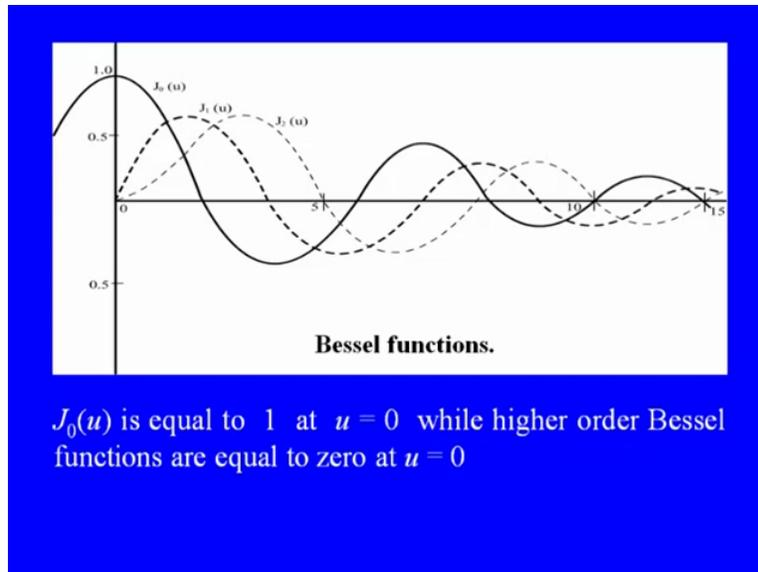
This shows a graphical representation of the various special functions.  $J_0$  of  $u$ ,  $u$  is the argument as a function of  $u$ ,  $J_1$  of  $u$ ,  $J_2$  of  $u$ . The main feature, this should be noted is, that these are oscillatory functions, then the oscillate, the amplitude goes on decreasing and  $J_0$  is = 1 at 0 argument at  $u$  is = 0 while higher order ones they all vanish at  $u = 0$ .
