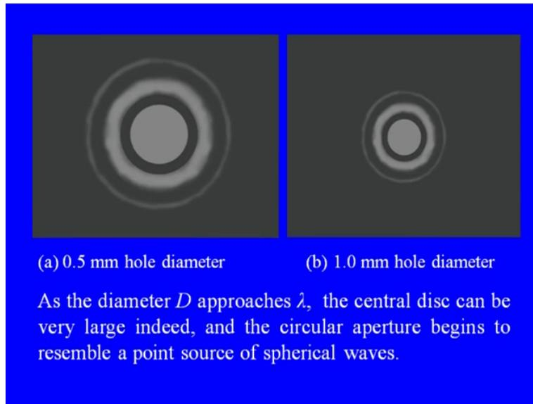
This picture shows for a aperture diameter of point 5 millimeter hole, a pattern will appear like this. For a 1 millimeter hole diameter, the main thing is as it  $D$  approaches  $\lambda$  becomes very very small the central disc can become very large indeed. And the circular aperture begins to resemble a point source of a spherical wave coming out in all directions, so the size of the disc becomes infinite.
