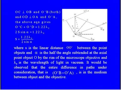
Therefore, drawing the line OC perpendicular to OB and O prime and OD perpendicular to both OA and O prime A, the above equation gives O Prime C + O Prime D = 1.22 Lambda. Therefore, we can we have 2S sin alpha = 1.22 lambda, so S will be = 1.22 lambda upon 2 sin alpha, where S is the linear distance O, O prime between the point objects and Alpha is the half the angle subtended at the axial point object O by the rim of the microscope objective and Lambda is the wavelength of light in vacuum.
