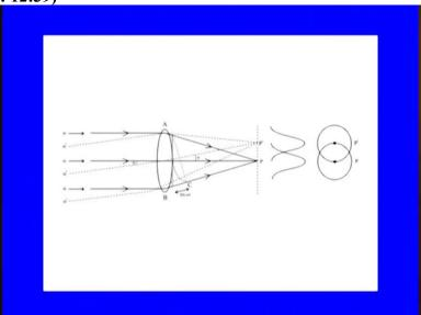
A beam of parallel rays from this object is incident normally on the objective. The ring supporting the lens as well as lens itself serves as a circular aperture and therefore from Fraunhofer diffraction pattern is produced in the focal plane of the lens. The refraction pattern of
