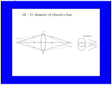
And the waves of light assumed to be of the same wavelength Lambda starting from self luminous point objects O and O prime are diffracted by the circular periphery of the lens. Therefore, a diffraction patterns corresponding to each object is formed in the focal plane of the objective. Each image is therefore a diffraction pattern consisting of a central bright desk bordered by alternate concentric circular dark and bright rings.
