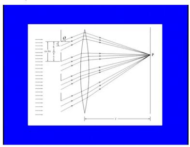
Each of width b and separated by equal optic spaces a as shown in this figure. This type of arrangement is known as diffraction grating. We will see that the diffraction pattern gets modified by the number of slits is increased beyond 2. Let a plane wave front of light of wave length lambda b incident normally on the slit as shown in this figure.
