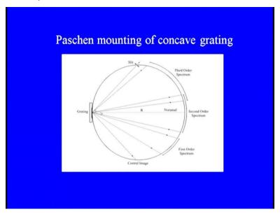
So if r is the radius of curvature of the spherical surface of the grating a circle of diameter R can be drawn tangent to the grating at its midpoint which defines the locus of points where the spectrum is in focus provided the source slit also lies on this circle as shown in this figure. This circle is called the Ronald circle and the mounting is known as Paschen mounting. So, till now we have discussed single slit, double slit and multiple slit diffraction pattern.
