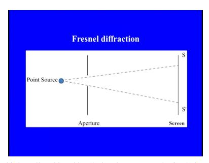
In the laboratory this is easily achieved by placing the source on the focal plane of a convex lens and placing the screen on the focal plane of another convex lens has shown in this figure.
