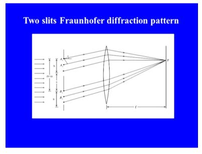
So, now let us discuss the diffraction pattern of double slit so here let us consider two parallel slits each of width b and separated by a opaque region of width a has shown in this figure. Now we will study in the diffraction pattern produced by two slits when a beam of monochromatic light of wavelength lambda is incident normally on the plane of the slits. Like single slit let us consider that both slit consists of a large number of equally spaced point sources.
