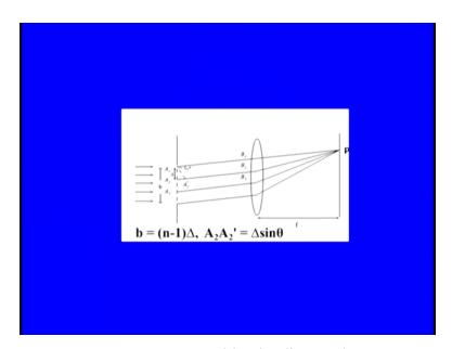
Let the point sources P at A1, A2, A3 so on and let the distance between two consecutive points be Delta as shown in this figure. Thus if there are n point sources on the slit then b will be = n - 1 Delta. We will now calculate the resultant field produced by these n sources at the point P which receive parallel rays making an angle theta with the normal to the slit. Since the slit actually consists of a continuous distribution of sources.
