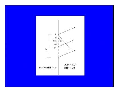
We now we divide the slit into two halves as shown in this figure consider two points A and A prime separated by a distance B by 2. Clearly the power difference between the disturbance emanating from A and A prime is B by 2 sine theta which in this case is lambda by 2. The corresponding phase difference will be Pi and the resultant disturbance will be 0. Similarly the disturbance from the point B will be cancelled by the disturbance reaching from the point B prime.
