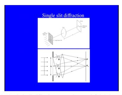
Now I will describe the single slit diffraction patterns due to an infinitely long slit of width b. Let us assume a plane monochromatic wave is incident normally on the slit. Now we want to calculate the intensity distribution on the focal plane of the lens l. When a plane wave front of monochromatic light of wavelength lambda is incident normally on the plane of the slit its size is limited at the instant it occupies the plane of the slit.
