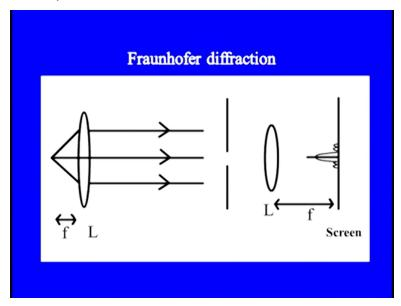
The two lenses effectively move the source and the screen to infinity because the first lens makes the light beam parallel and the second lens effectively makes the screen receive a parallel beam of light.
