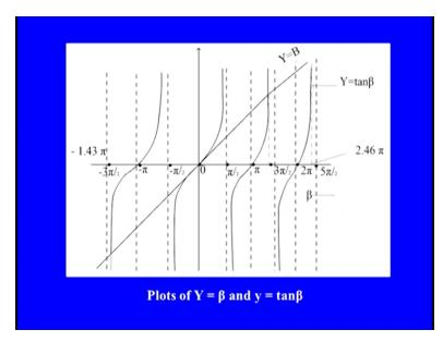
The roots of this equation can be found by determining the position of intersections of the curves Y = beta and y = tan beta as shown in this diagram. The intersections occur and beta = 0 and beta = 1.43 Pi and beta = 2.46 by etc. The root beta = 0 correspond to the central maxima and for this we have I = I naught. The other roots like beta = 1.43 Pi beta = 2.46 Pi etc give the position of first Maxima, second Maxima so on.
