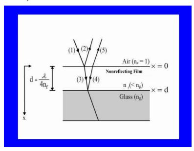
Bottom is the glass, it is coated by a non reflecting film of reflective index nf which is less than ng and the top is naturally air, refractive index is 1, nf is intermediate between na and ng. The thickness of the non reflecting film is d is = lambda upon 4 and it is called lambda by 4n for film and thickness of this film is d which is = lambda by 4 and m.
