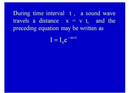
During the time interval t, a sound wave travels a distance x given by v into t and the preceding equation may now be written as I = I naught e raise to the power - mvt.
