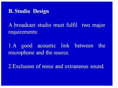
A broadcast studio must fulfill two major requirements: A good acoustic link between the microphone and the source and exclusion of noise and extraneous sound.
