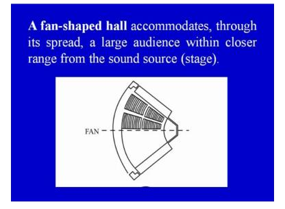
A fan shaped hall accommodates through its spread a large audience within closer range from the sound source from the stage.
