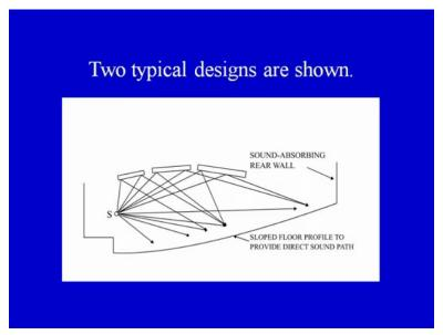
Two Typical designs are shown for the floor profiling and for the design of the ceiling. **(Refer Slide Time: 29:30)**
