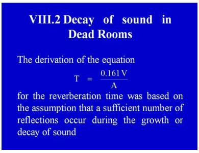
Now, the derivation of the equation t = 0.161 V by A for the reverberation time was based on the assumption that a sufficient number of reflections occur during the growth or decay of sound.
