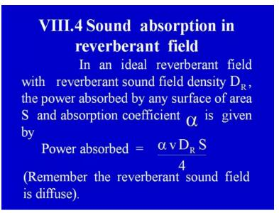
Let us now consider Sound absorption in reverberant field. In an ideal reverberant field with the reverberant sound field in density DR, the power absorbed by any surface of area has absorption coefficient alpha is given by the power absorbed is given by alpha into v into DR times S divided by 4. Remember, the reverberant sound field is the diffuse phase.
