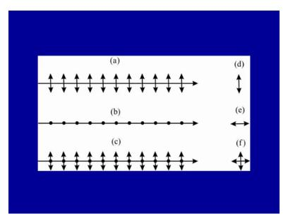
This figure shows a pictorial representation of side views a, b and c and end views d, e, f of being polarized and unpolarized ordinary light beams.
