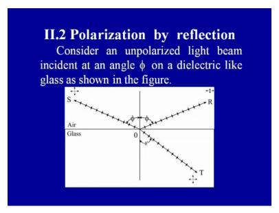
Consider an unpolarized light beam incident at an angle Pi, on a dielectric like glass as shown in the figure.
