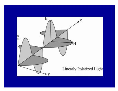
This picture shows the electric and magnetic fields of an x polarized light, propagating in the z direction. The light shaded region depicts oscillations of electric field along the x axis.
