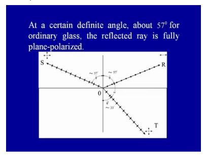
At a certain definite angle of about 57 degrees for ordinary glass, the reflected ray is fully plane-polarized. It was Brewster who first discovered that at the polarizing angle Phi bar.
