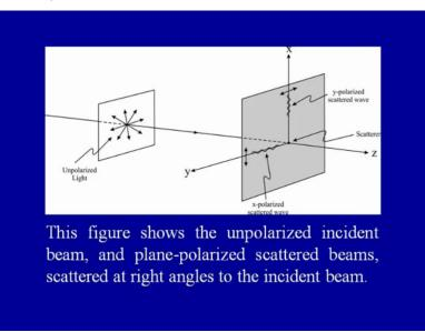
This figure shows the unpolarized incident beam and plane polarized is scattered beams is scattered at right angle to the incident beam. The incident wave is propagating along the z direction then the scattered wave along the y direction is x polarized.
