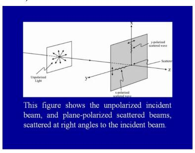
If the incident beam is plane polarized with its electric vector along the x direction, then, there will be no scattered light along the x axis.
