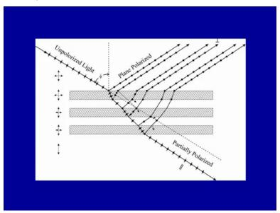
The figure shows the arrangement of pile of plates. The marking is given from the left of the figure with shortening horizontal arrows indicate that the transmitted beam is becoming more and more plane polarized.
