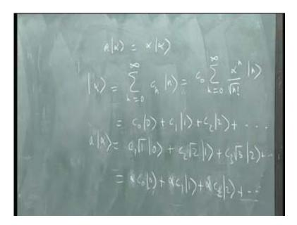
This is equal to a summation from n=0 to infinity, there is a coefficient  $c_0$  that comes out and then there is an alpha to the n acting on n over square root of n factorial. So we have a state. What are the allowed values of alpha? It can be any complex number. So it has a double continuous infinity of eigenvalues. All numbers in the complex plane are eigenvalues of the annihilation operator a. and they have corresponding normalizable eigen states. Let's normalize them.
