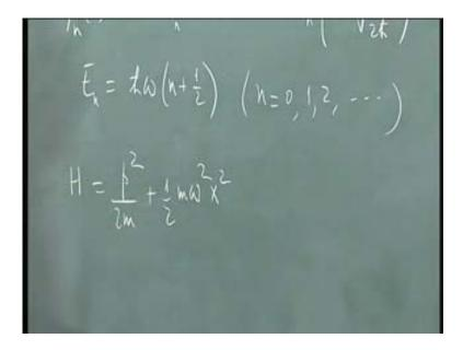
Now recall that the Hamilton for this problem was p squared over 2 m + 1 half m omega squared x squared where x and p are operators; the position momentum operators. apart from these coefficients its quadratic in x and its quadratic in p. so there is a complete symmetry between the position space wave functions and the momentum space wave functions in this case because what appears here is completely symmetric in x and p.
